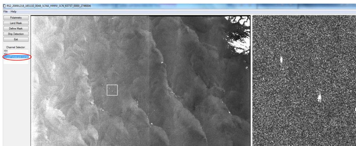
Figure 3.13 The location where it is possible to choose the fused polarimetric “channel” (see red circle to the left).
