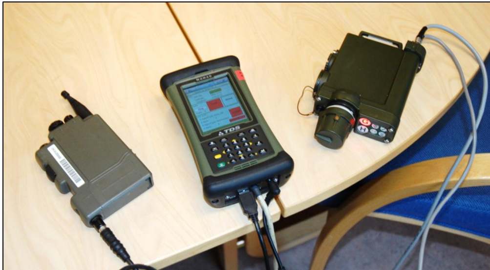
Figure 2.1 A Lightweight Chemical Detector (LCD) showing a nerve agent alarm (right) connected to a radio (left) and a personal data assistant (middle) (Photo: FFI).
