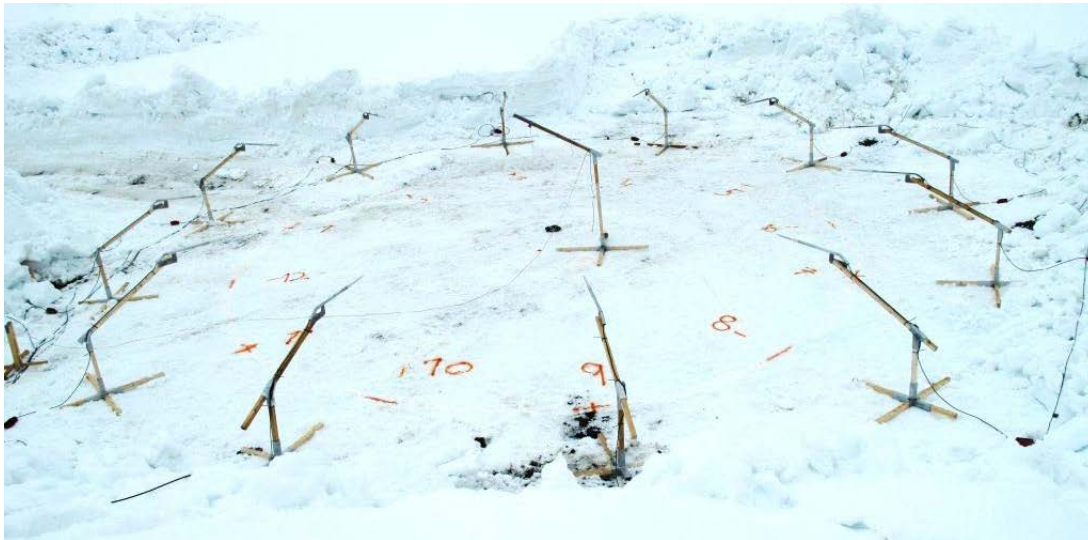
Figure 3.2 Picture from the misalignment tests showing the circular setup of the pencil probes mounted on the wooden stands, with a similar stand for the explosive charge at the centre.
