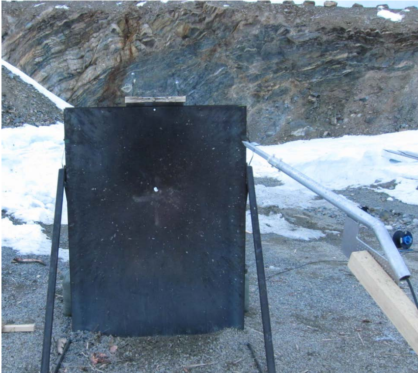
Figure 1.1 Blast pencil probe pointing towards a virtual blast source on top of a steel plate.
