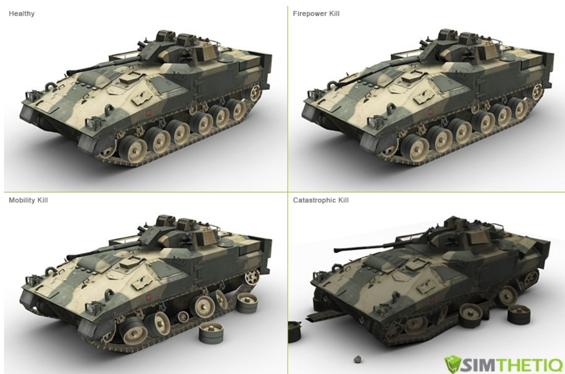
Figure 3.20 Examples of 3D models of a combat vehicle with various damage states (healthy, firepower kill, mobility kill, catastrophic kill) (Simthetiq).
