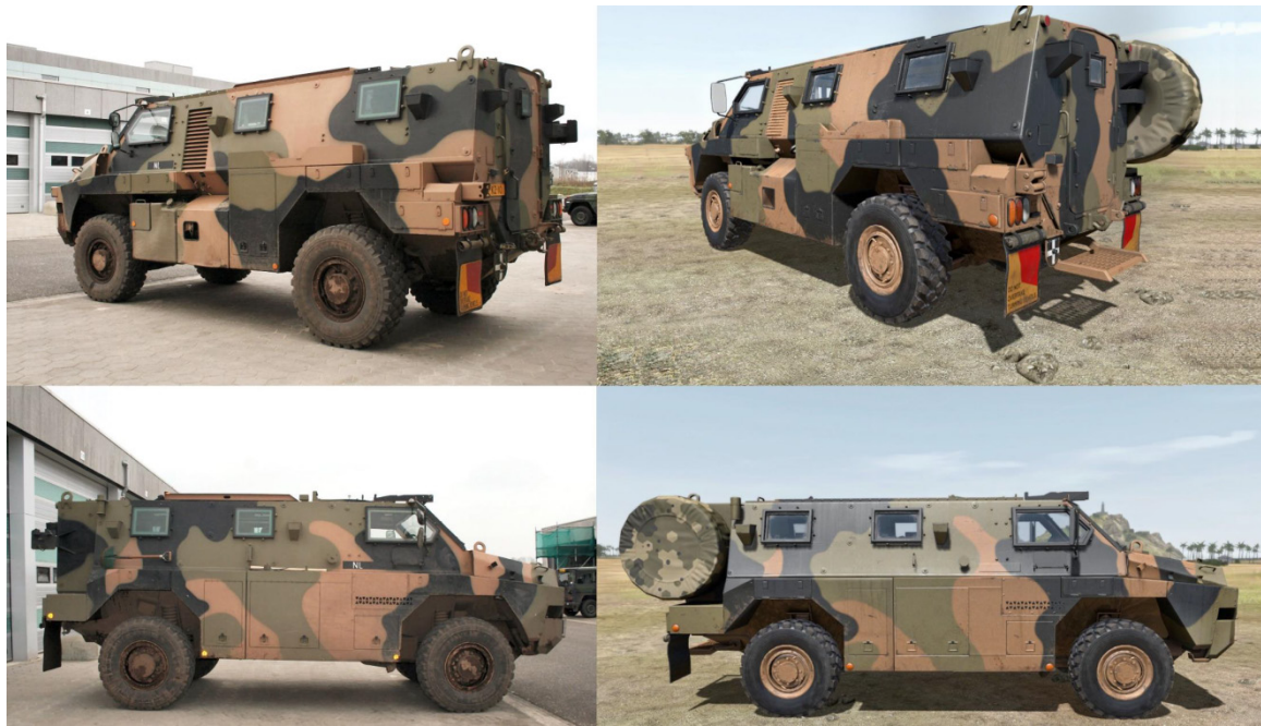
Figure 3.18 Example of a high-resolution, high-fidelity 3D model of a combat vehicle in VBS (to the right) alongside the real-world vehicle (to the left) (Bohemia Interactive Simulations).
