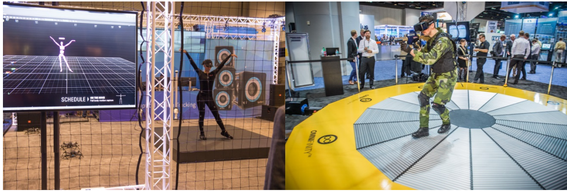
Figure 3.4 Example of a body tracking system (to the left), and a virtual dismounted soldier simulator using an omnidirectional treadmill (to the right) (Interservice/Industry Training, Simulation and Education Conference).
