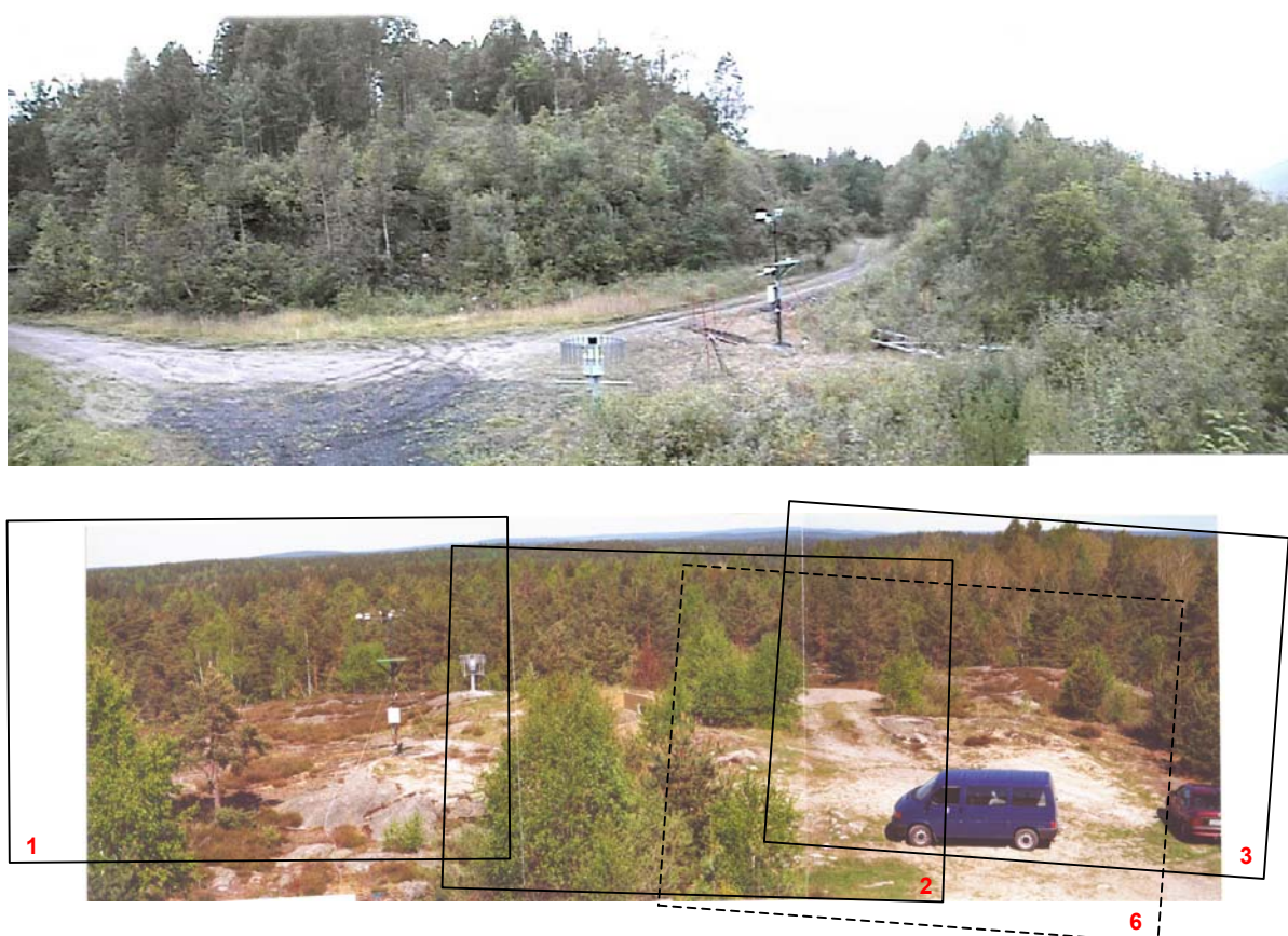
Figure 2.2 Pictures taken from the camera mast at Bardufoss (top) and Rygge. Fields of view of the thermal camera (1 to 3 and 6) are given for Rygge. The meteorology mast and precipitation sensor can be clearly seen.
