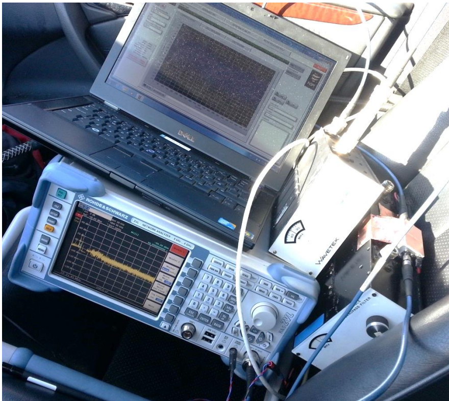
Figure B.2 The measurement system in action with laptop, filters, spectrum analyser, and cables.
