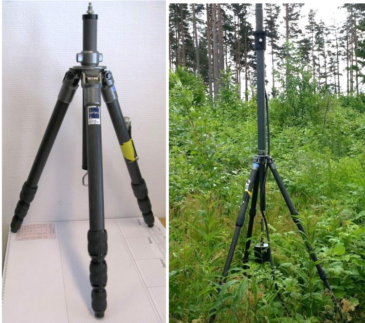
Figure B.3 The Gitzo G1228Mk2 tripod. - To the left, the unmodified tripod. - To the right, the tripod during measurement, with counterweight, rod, and antenna adapter.
