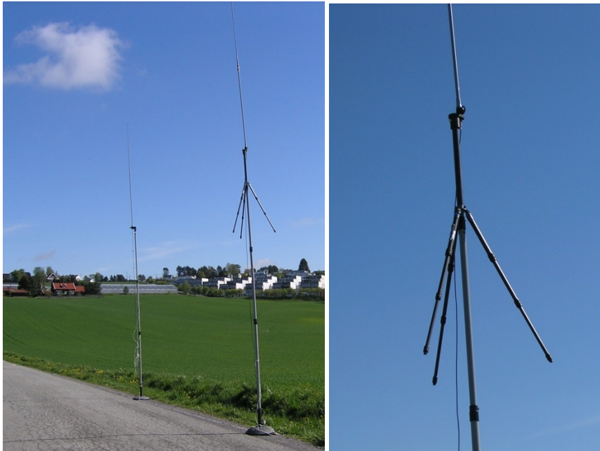
Figure D.8 Antenna test range. Measuring the tripod's influence on the Comrod VHF30108VM's gain.
