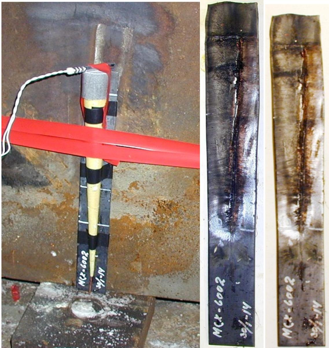
*Figure 3.5 Setup and the witness plate for testing of conical charge cast 6/14 with MCX-6002 CH 6080/13 composition.*
