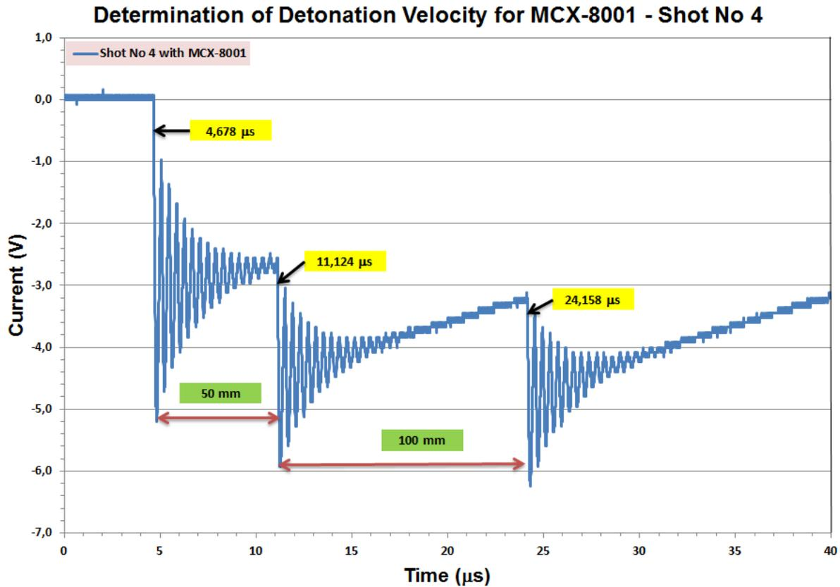
Figure 3.21 The figure shows the arrival time of the detonation front for each pin and the distance between pins.
