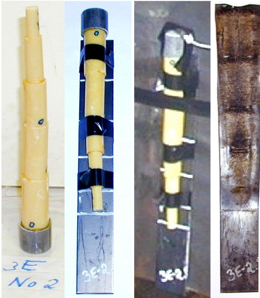
*Figure 3.2 Different pictures: from left the test item after being glued together, next after the test item been assembled on the witness plate, setup for firing and to the right the witness plate after firing.*
