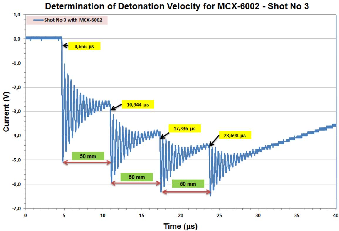
Figure 3.14 The figure shows the arrival time of the detonation front for each pin and the distance between pins.
