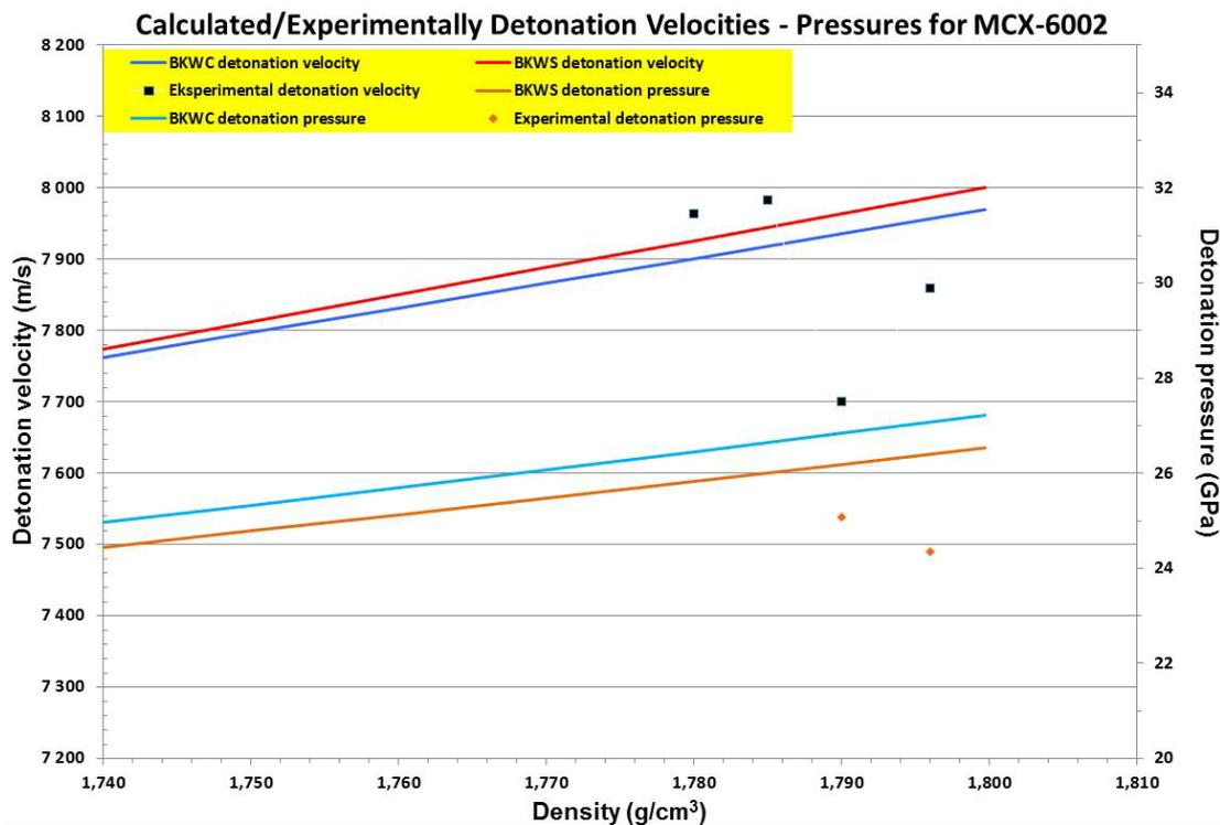
Figure 3.27 Calculated and measured detonation velocities and pressures for MCX-6002 as function of density.
