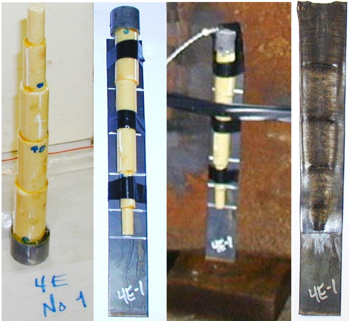
Figure 3.8 Different pictures: from left the test item after being glued together, next after the test item been assembled on the witness plate, setup for firing and to the right the witness plate after firing.
