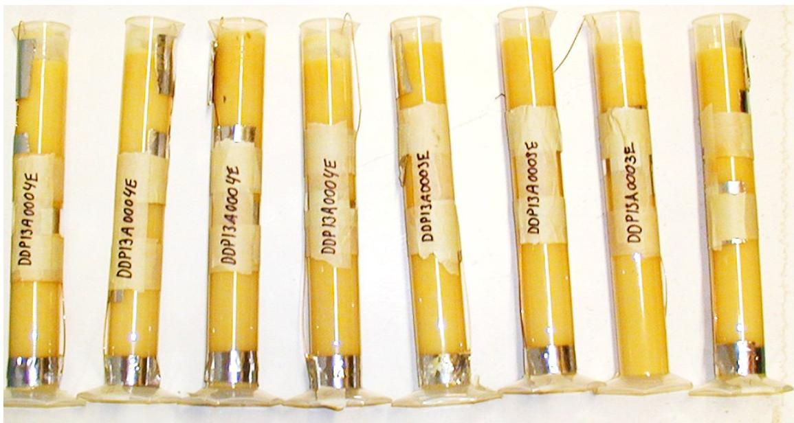
Figure 2.1 Filled moulds, 4 with MCX-6002 (left) and 4 with MCX-8001 (right) compositions after the melt had solidified.
