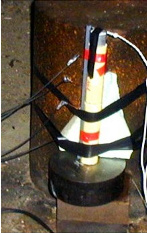
Figure 3.18 Test setup for the first firing with MCX-8001 Lot DDP13A0004E.
