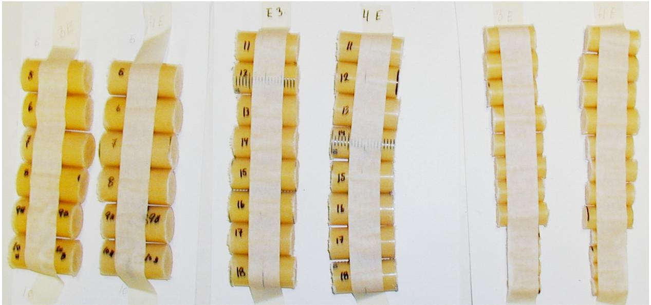
Figure 2.6 Pictures of the smaller charges casted for critical diameter and mechanical testing. Charges marked with 3E contain composition MCX-6002 and 4E contain composition MCX-8001.
