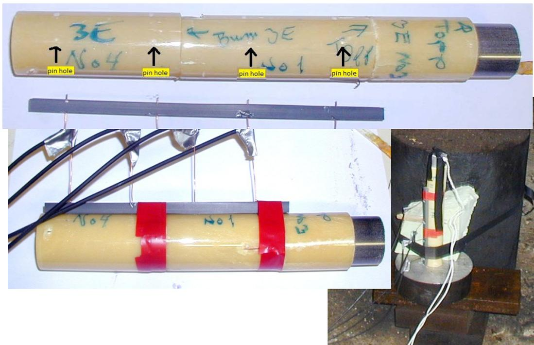
Figure 3.13 The first picture shows where the ionization pins were positioned. The second picture shows the charge after the pins was set in and the right picture shows the setup for testing.
