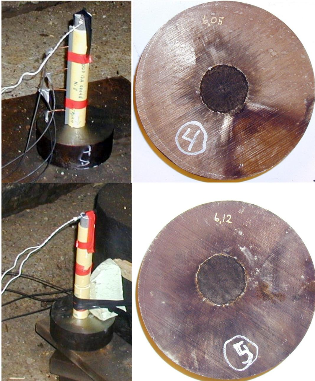
Figure 3.26 The Figure shows the setup and Dent plates after firing for the two tested charges containing the MCX 8001 composition Lot DDP13A0004E.
