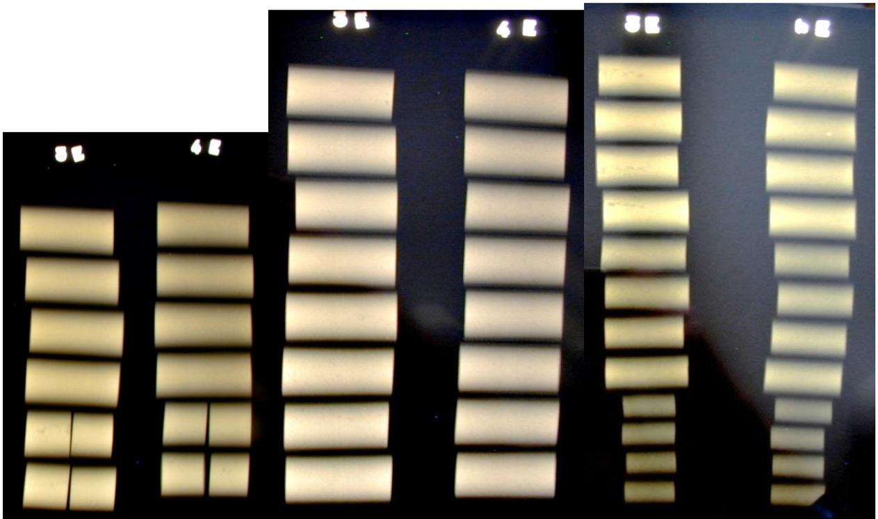
Figure 2.7 Pictures of X-ray films of the items in Figure 2.6. Charges marked with 3E contain composition MCX-6002 and 4E contain composition MCX-8001.
