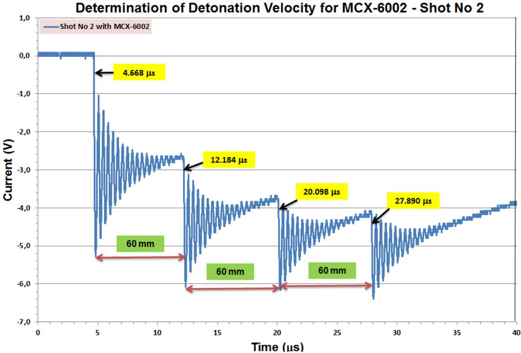
Figure 3.12 The figure shows the arrival time of the detonation front for each pin and the distance between pins.
