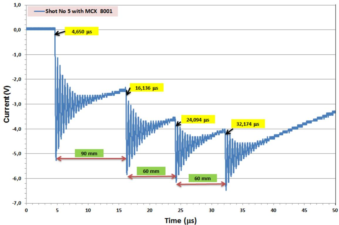
Figure 3.23 The figure shows the arrival time of the detonation front for each pin and the distance between pins.
