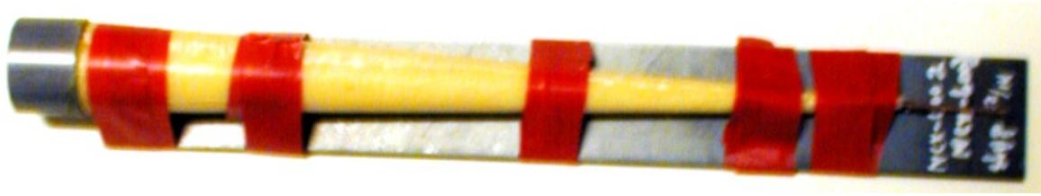
Figure 2.13 Picture of the MCX-6002 CH 6080/13 conical charge cast No 12/14 after been assembled on the witness plate.
