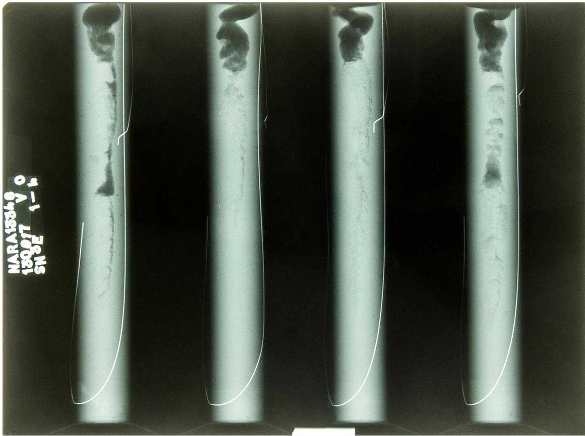
Figure 2.2 The figure shows the X-ray picture of the four tubes filled with MCX-6002 composition.
