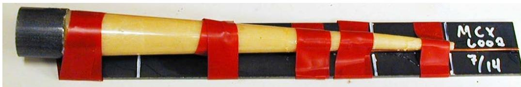
Figure 2.9 Picture of the MCX-6002 CH 6080/13 conical charge cast No 7/14 after been assembled on the witness plate.
