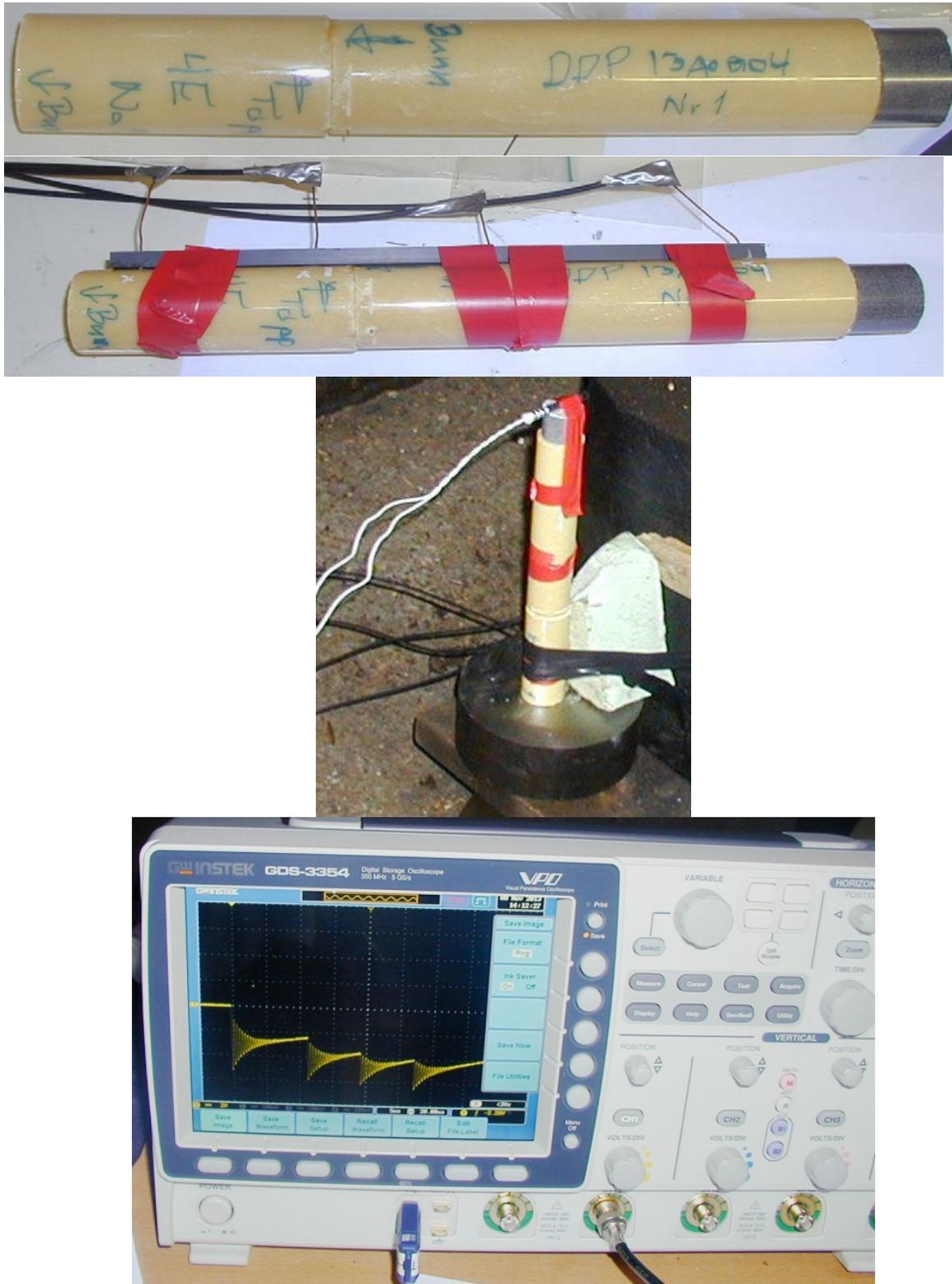
Figure 3.22 The two first pictures show the test item without and with the ionization pins follow by the test setup and the scope with the obtained registration.at the bottom
