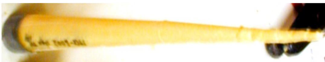
Figure 2.12 Picture of the MCX-6002 CH 6080/13 conical charge cast No 12/14 after been released from mould and added booster.
