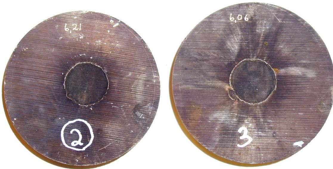
Figure 3.24 The Figure shows the setup and the Dent plates after firing for the two tested charges containing the MCX 6002 composition.
