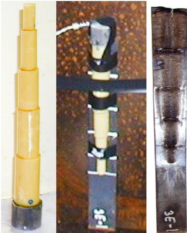
Figure 3.1 Different pictures of the test item used to determine critical diameter: from left after being glued together, test setup for firing and right the witness plate after firing.
