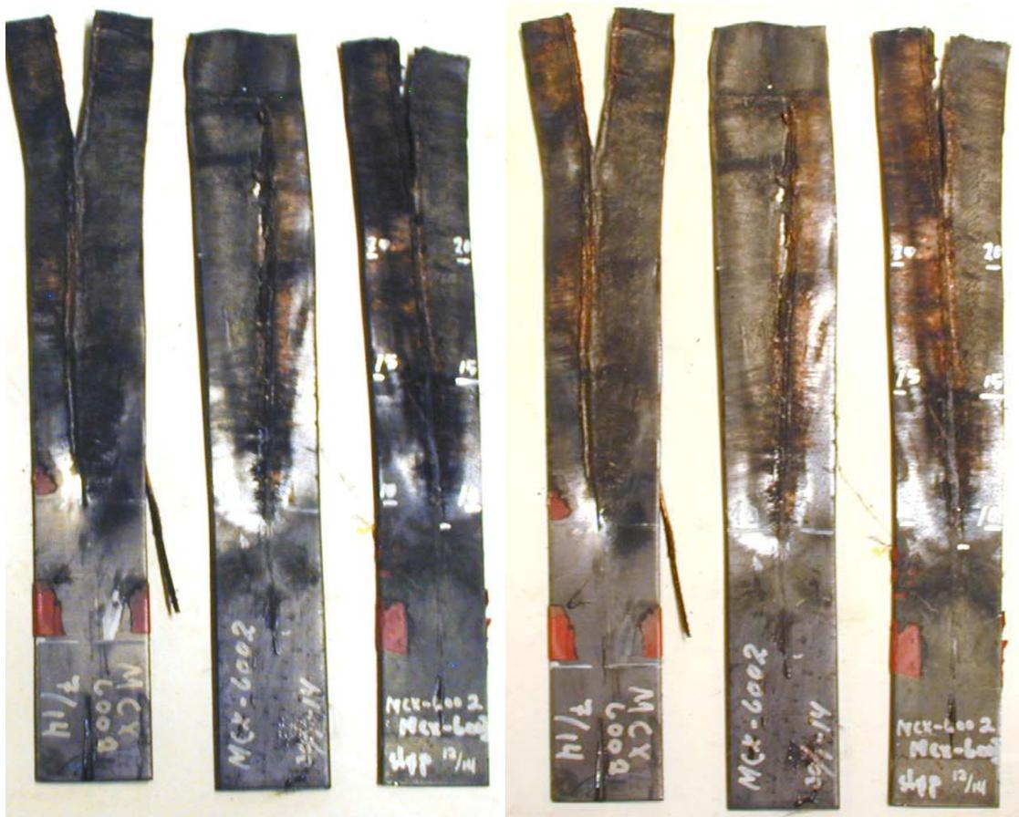
Figure 3.7 The figure shows two pictures of the witness plates for the three firing with conical charges containing MCX-6002 CH 6080/13 compositions.
