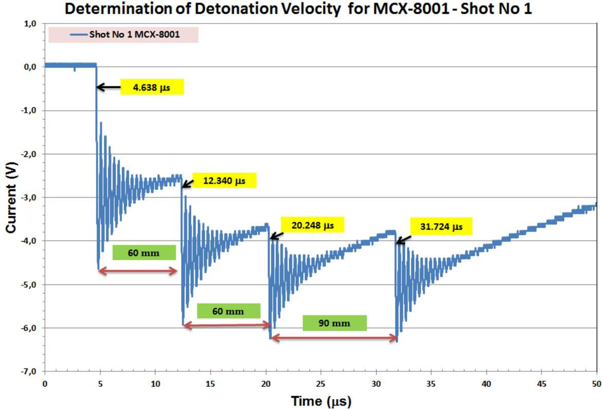
Figure 3.19 The figure shows the arrival time of the detonation front for each pin and the distances between the pins for shot No 1 containing MCX-8001.
