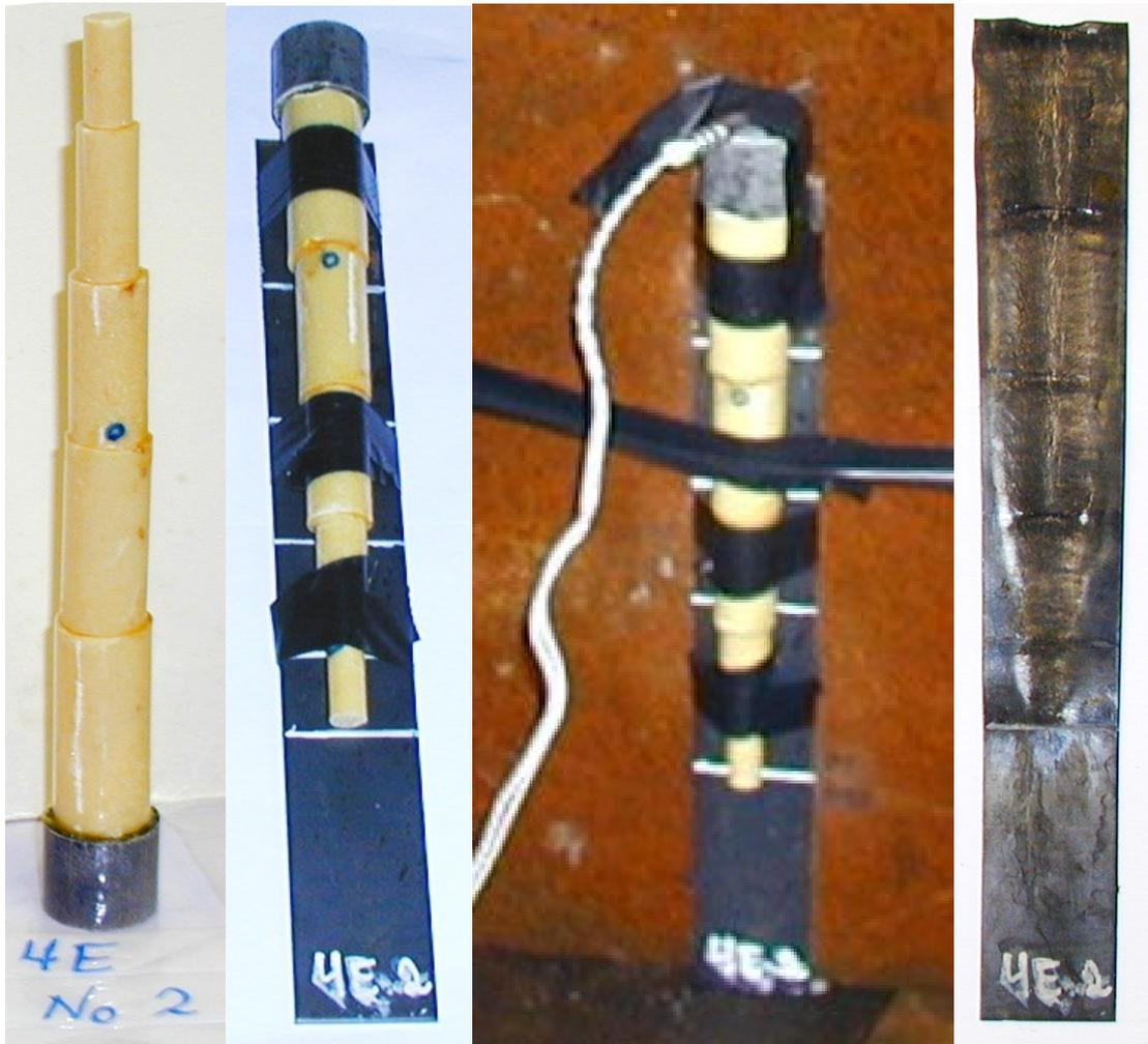
*Figure 3.9 Different pictures: from left the test item after being glued together, next after the test item been assembled on the witness plate, setup for firing and to the right the witness plate after firing.*
