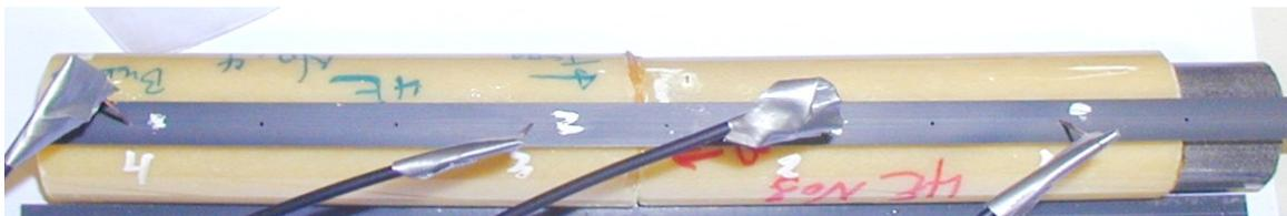
Figure 3.17 Picture of the test item with the ionization pins.
