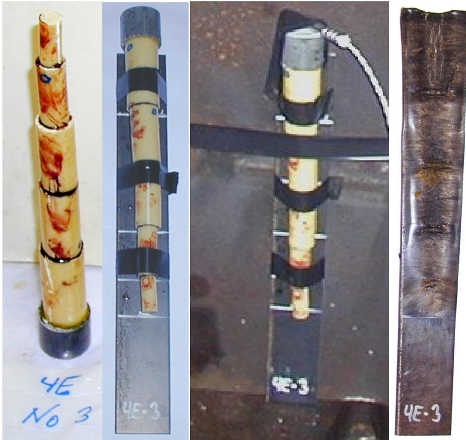
Figure 3.10 Different pictures: from left the test item after being glued together, next after the test item been assembled on the witness plate, setup for firing and to the right the witness plate after firing.
