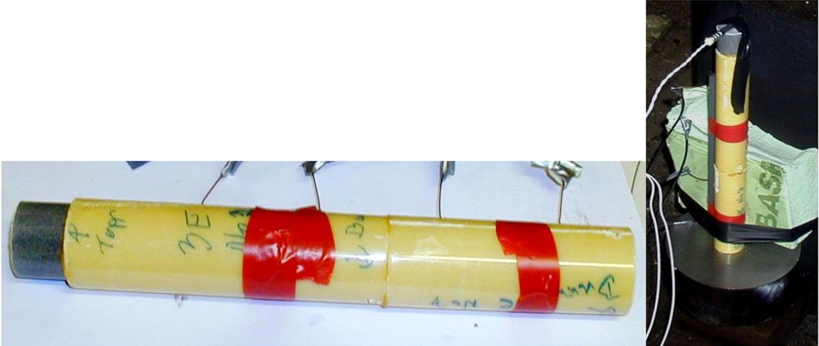
Figure 3.11 Left picture shows the charge after the ionization pins had been positioned. Right picture shows the charge setup for firing.
