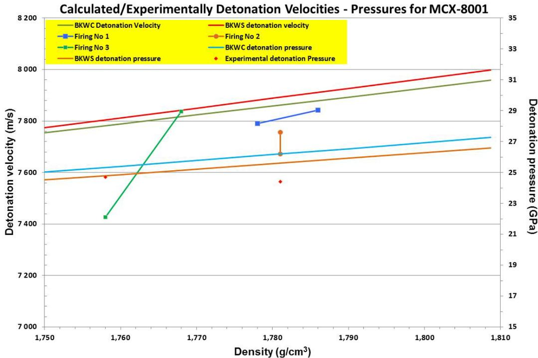
Figure 3.28 Calculated and measured detonation velocities and detonation pressures for MCX-8001 as function of density.
