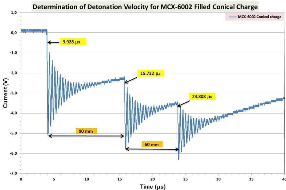
Figure 3.16 The figure shows the arrival time of the detonation front for each pin and the distance between pins for the conical firing of MCX-6002 CH 6080/13.
