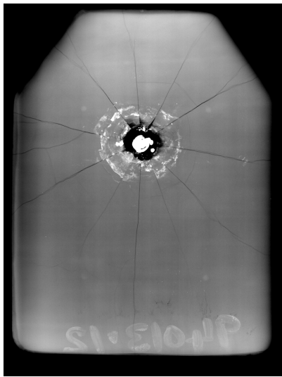
(a) Cracks in a ceramic without cover tile after one shot.
