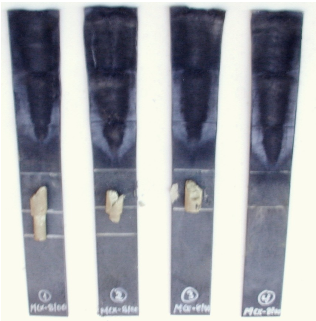
Figure 3.5 Pictures of the witness plates including recovered explosives for firings with MCX-8100 test items for determination of critical diameter.
