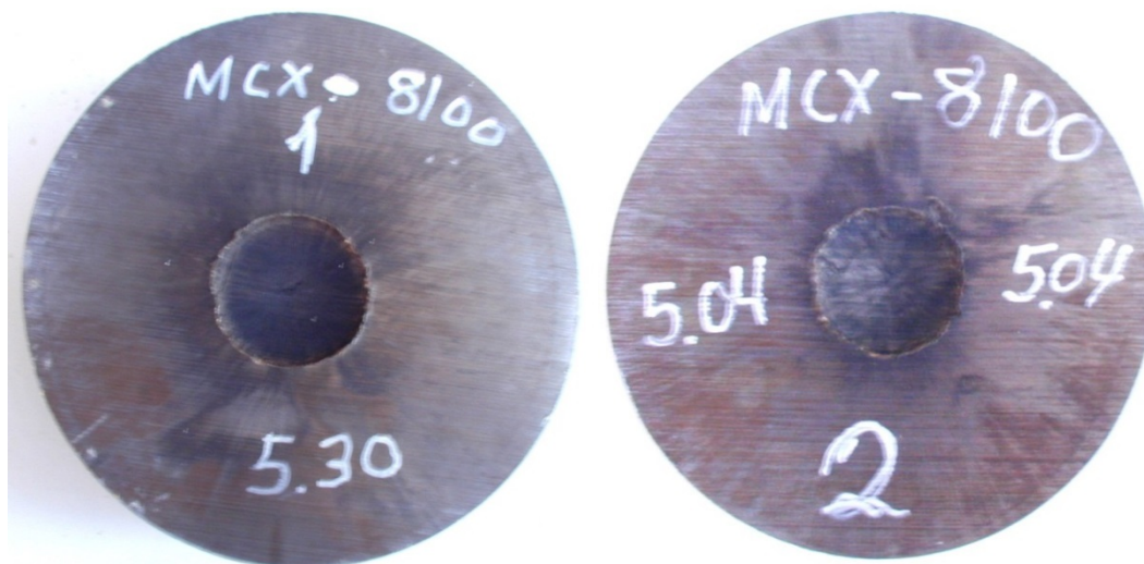
Figure 3.10 The Figure shows the Plate Dent witness plates for the two tested charges containing the MCX 8100 composition.
