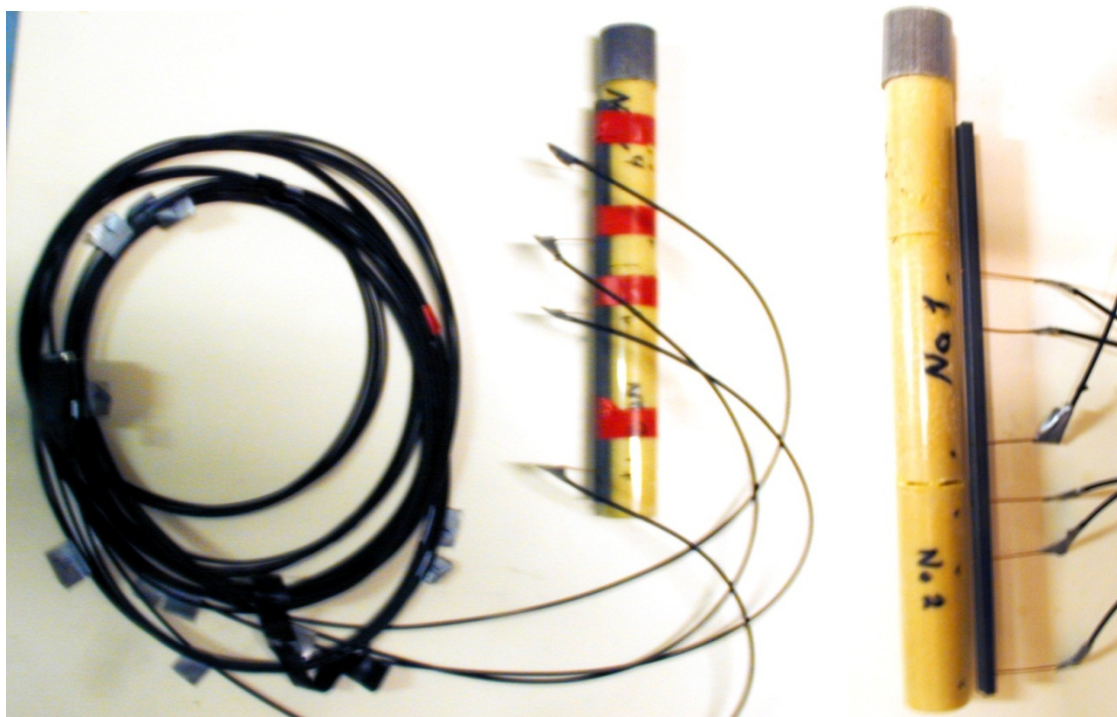
Figure 2.4 The test item used for determination of detonation velocity.
