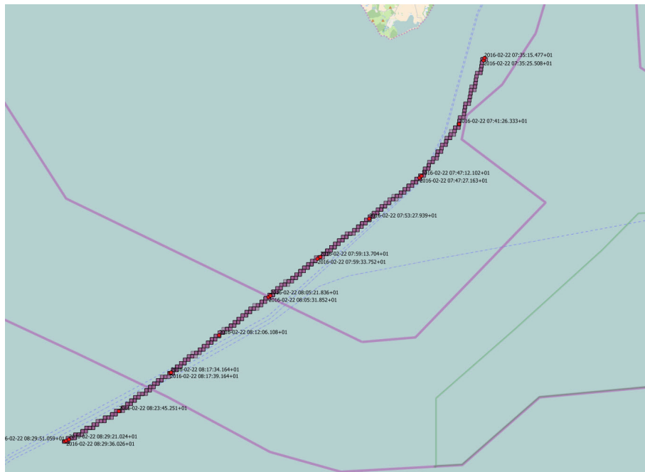
Figure 3.7 Each position is tied (moved) to the closest grid cell center. The cell square is drawn to show its extent (coverage).
