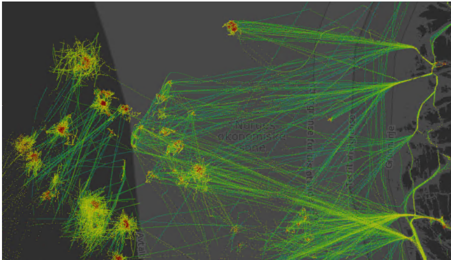
Figure 4.15 Density map showing January of 2015 with only platform supply offshore ship type, classification B21A2OS, Northern Norwegian Sea. Scale factor 1.
