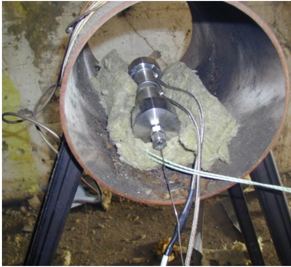
Figure 2.7 Picture of the test item with two heating elements and three thermocouples.
