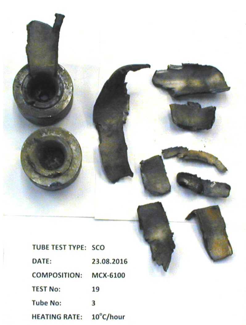
Figure 3.10 Picture of recovered fragments of tube No 3.
