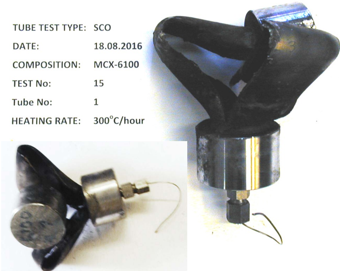
Figure 3.4 Recovered test item rest from test of tube No 1 filled with MCX-6100 CH 6027/14.
