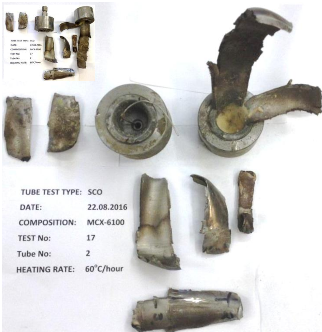
Figure 3.7 Picture of the recovered items from tube No2 filled with MCX-6100 CH 6027/14.
