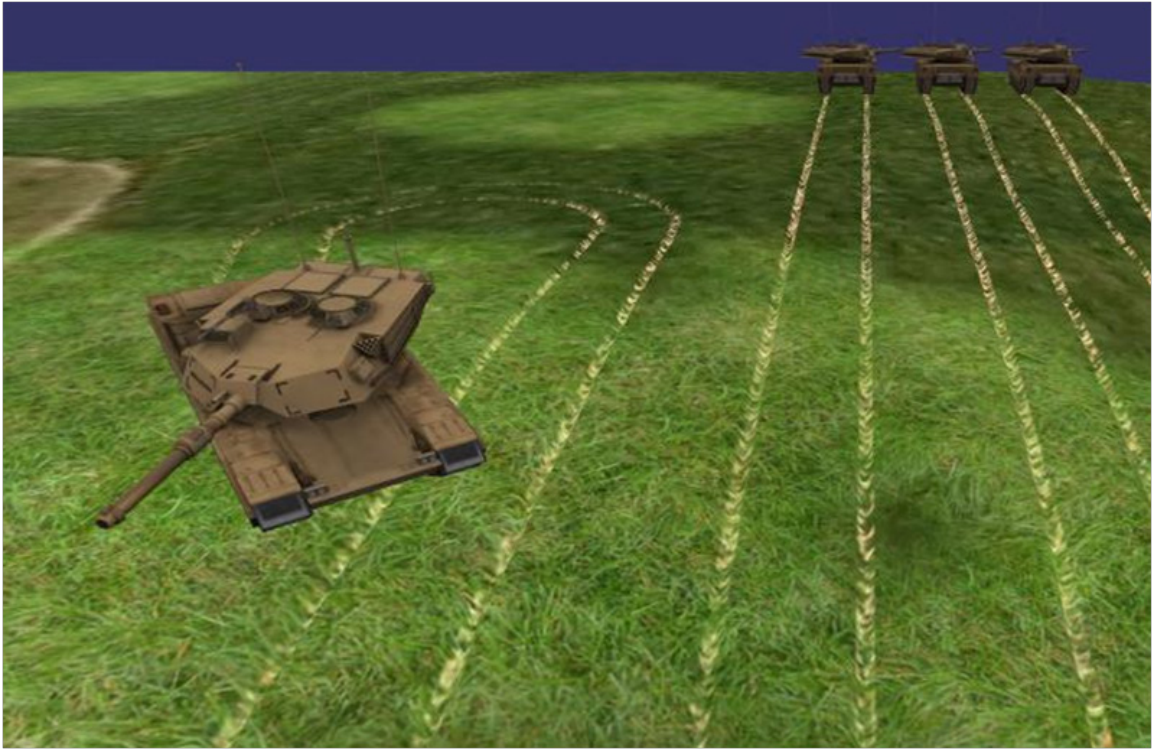
Figure 7.4 Armored vehicle tracks. Both elevation data and textures encode the tracks.
