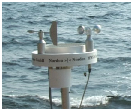
Figure C.7 Reinhardt meteorology station near the waterline.
