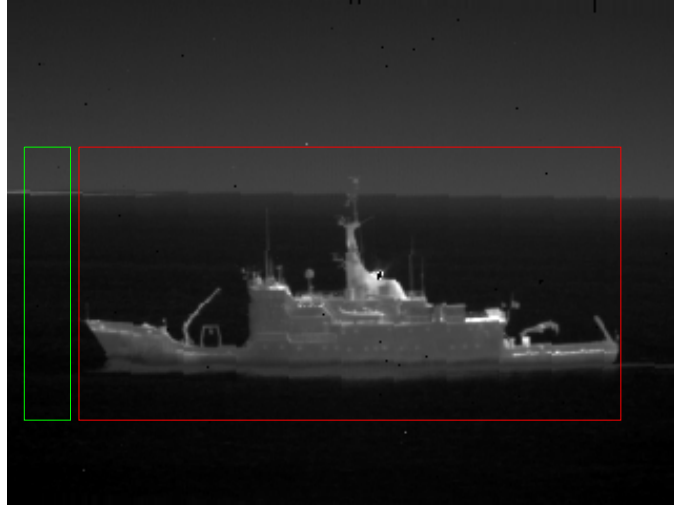
Figure 2.1 Illustration of scene with target area marked with red, and background area marked with green. Illustration image recorded by NRL with Indigo Merlin (MW) IR camera.
