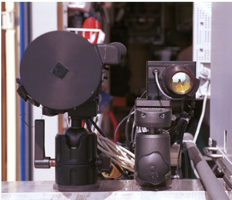
Figure 3.4 Amber Sentinel (LW) camera to the left, and Inframetrics MilCam (MW) camera to the right.
