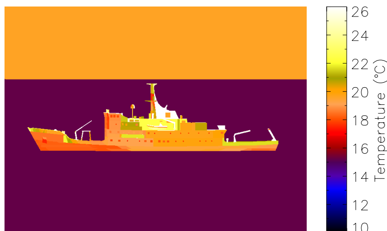
Figure 4.17 A temperature map of the scene for run 8. The aspect and the color coding is the same as in figure 3.12. Note that calculated temperatures are shown, not equivalent temperatures.
