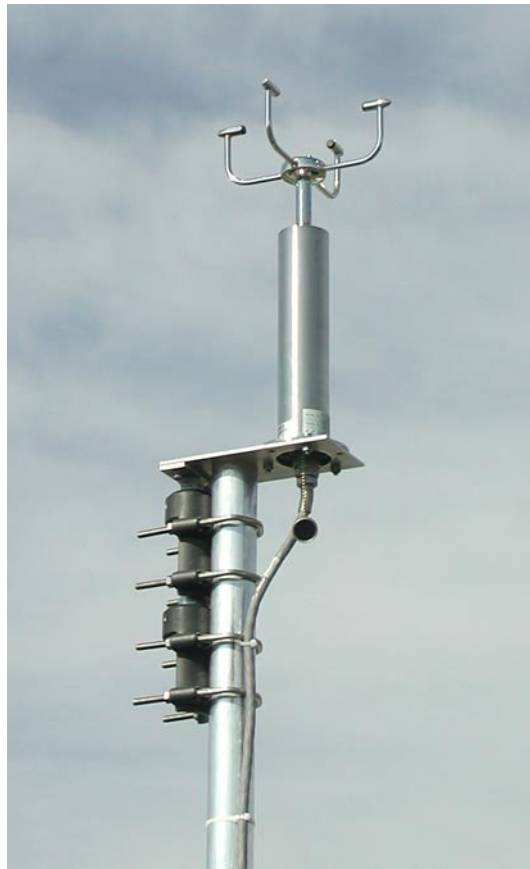
Figure C.2 Sensor for wind speed and direction measurements. This is an ultra-sonic wind sensor without any moving parts.
