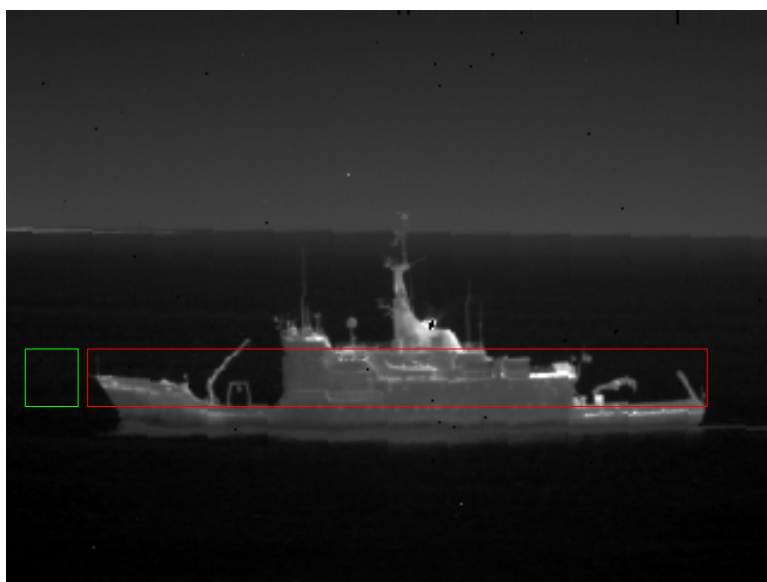
Figure 4.8 The red box defines the superstructure region used in the division of the ship in three parts. The hull is below this region while the funnel is above the superstructure region.
