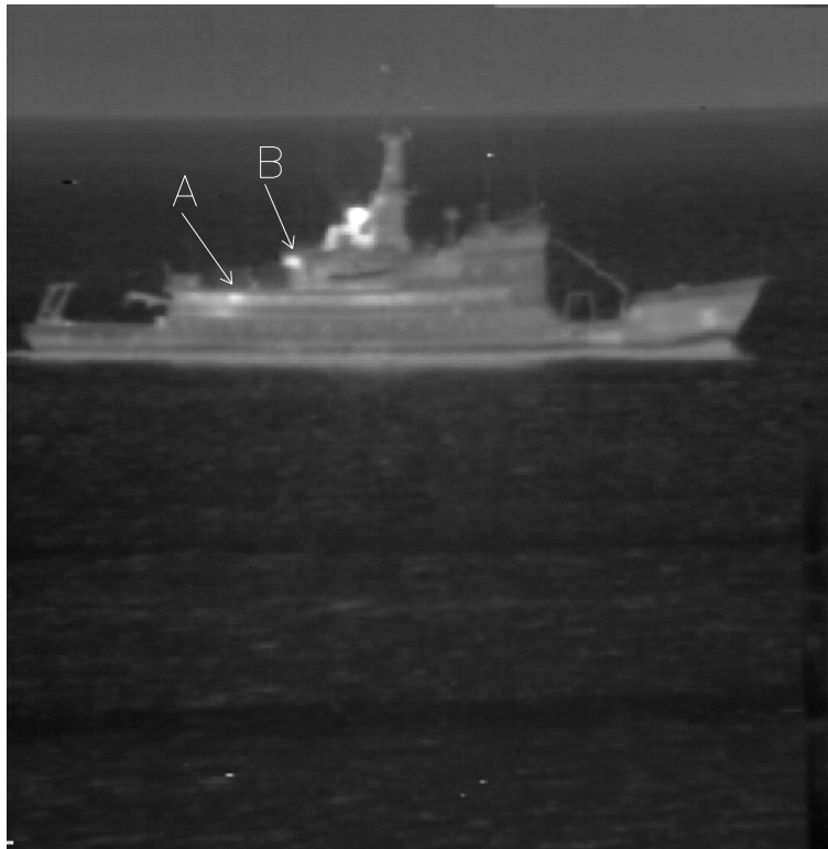
Figure 3.19 IR image (MW) of CFAV Quest, distance 1056 m, run 34, 23:37:52 (UTC). A and B indicates hot areas that don't have counterparts on the port side.
