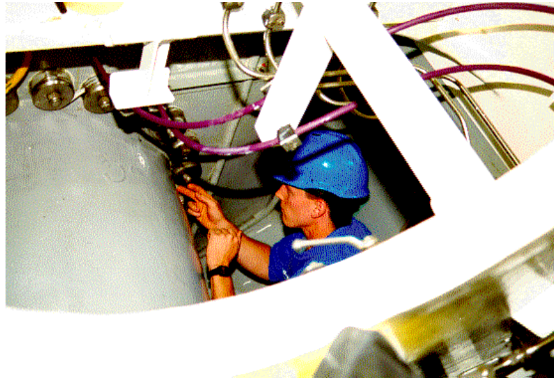
Figure 3.3 From mounting of sensors on the water jet tube
