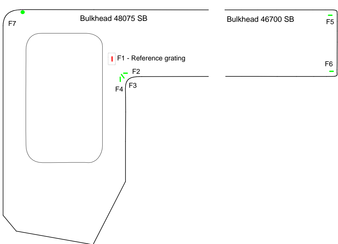
Figure 3.9 Approximate positions of the seven sensors in array F, details in Appendix A
