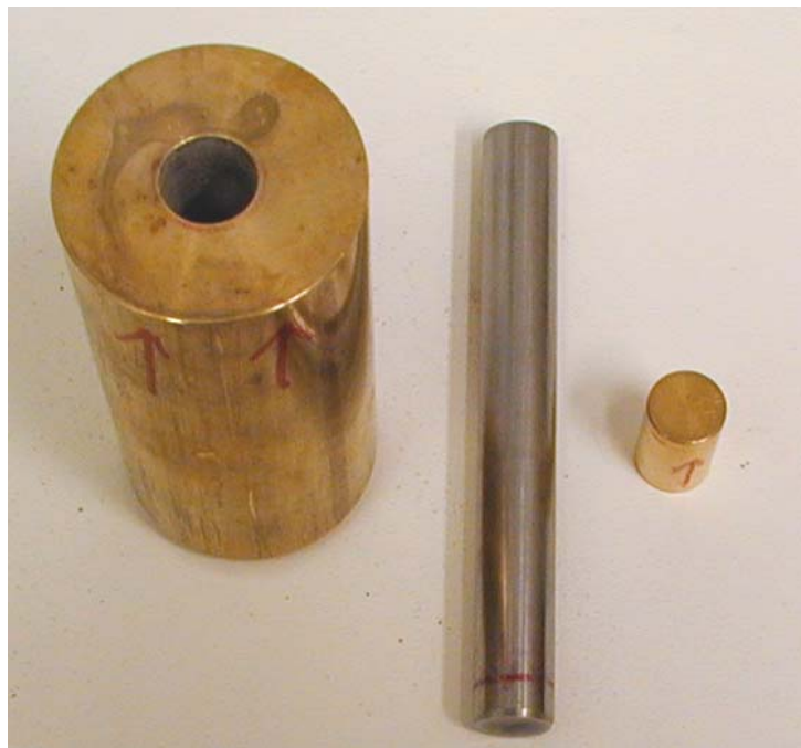
Figure 2.3 Picture of press tool used to produce pellets with density up to 1.79 g/cm 3 .
