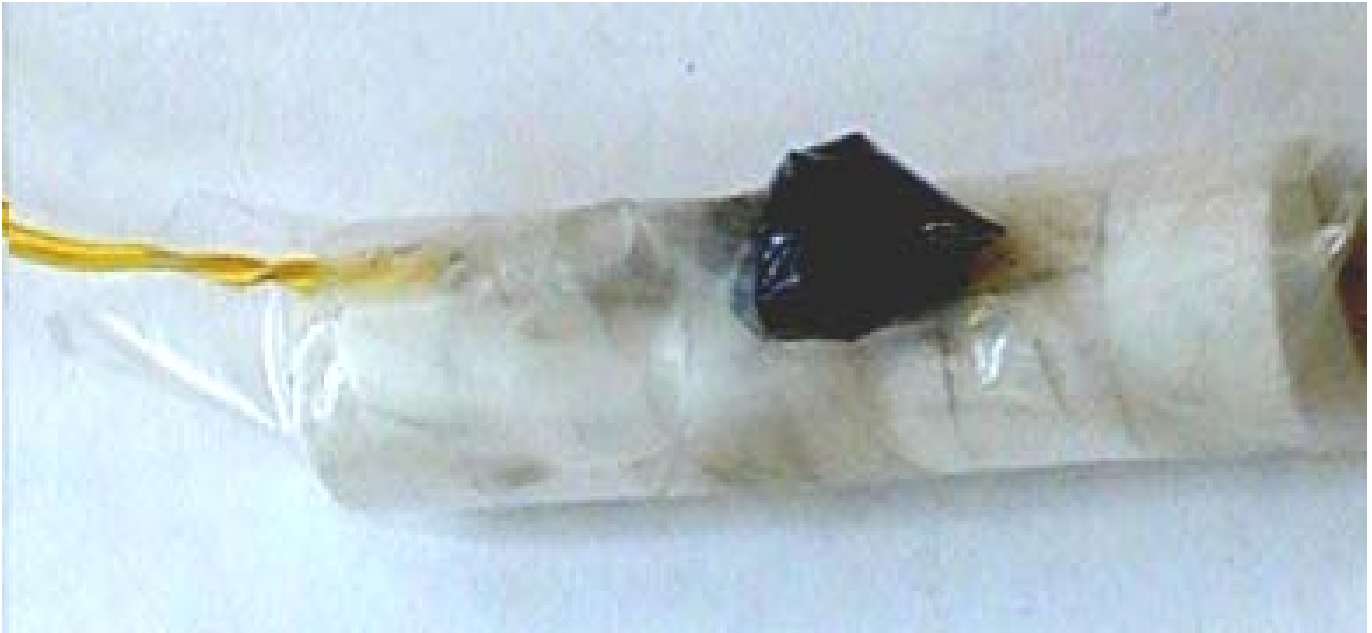
Figure 3.20 Picture of the orientation of the pellets and ignition device before firing.
