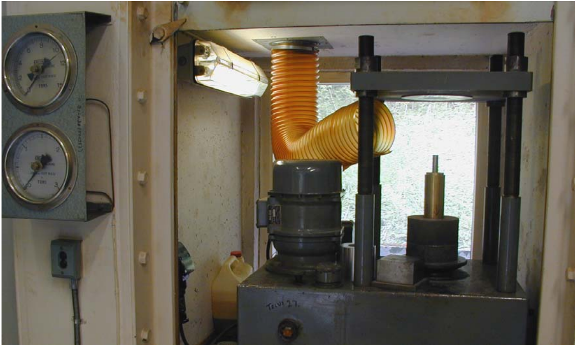
Figure 2.2 Picture of the press used to produce pellets with density up to 1.79 g/cm 3 .
