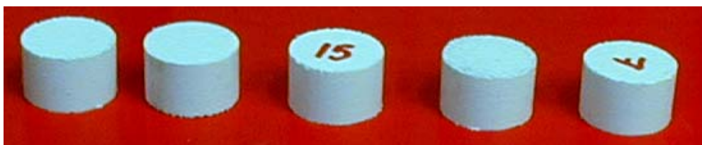
Figure 3.19 Pressed PBXN-5 pellets for testing in Closed Vessel.
