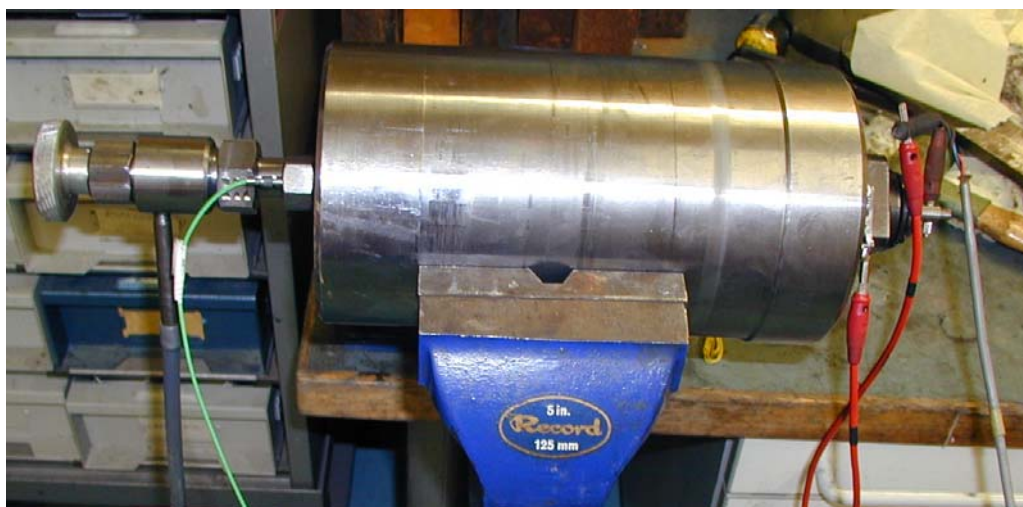
Figure 2.1 A picture of the 150 cm 3 Closed Vessel used for the experimental testing.
