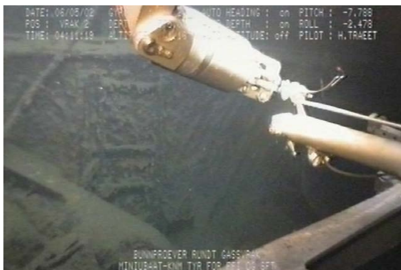
Figure 2.13 Water samples were collected using a Nansen water-sampling device. This picture is from wreck no 5
