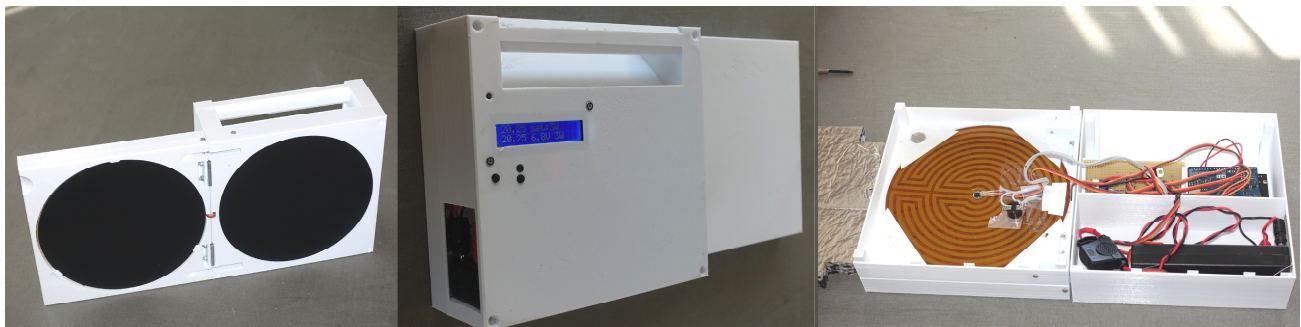
Figure 3.2 Multi-source blackbody with 3D printed casing. Left: Front side with two blackbodies facing the sensor, one at ambient temperature (left side) and one with a foil heater (right side). The hinged cabinet can be closed so that the blackbody surfaces are protected during transport and storage. Center: Back side with a simple LCD display and buttons. On the side of the cabinet is the battery compartment opening. Right: Interior of the main cabinet, showing the foil heater and temperature sensor on the left, with foam insulation removed. On the right is the microcontroller with LCD "shield" and a board with the few extra components needed. Here the battery compartment holds a 7.2V, 5Ah Li-ion battery.
