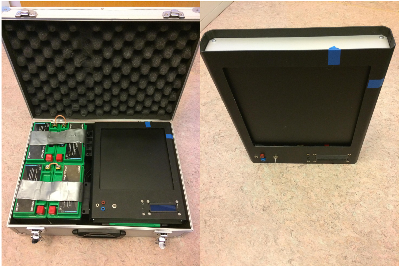
Figure 3.1 Blackbody with homogeneous output, seen as a part of a kit (left) and free-standing (right). A display and a simple button user interface is seen lower right. As can be seen, there are two pairs of batteries in the kit. The charging time for the batteries is shorter than the operation time during one discharge at 100°C, so the blackbody could in principle be operated almost continuously on batteries.
