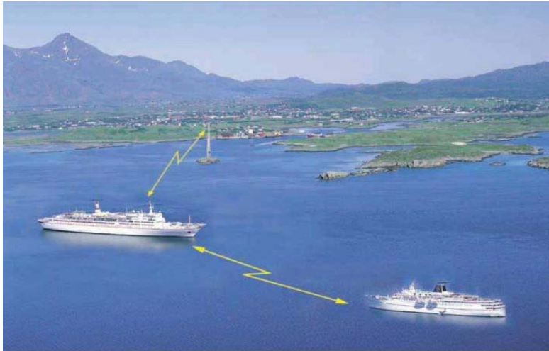
Figure 2.1 The AIS ship-to ship and ship-to-shore concept (Courtesy of Kongsberg Seatex).
