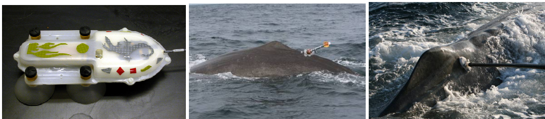
DTAG (left), and deployment of the tag to sperm whales using the ARTS system (middle) and a hand held pole (right).
