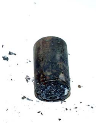
Figur 3.8, utbrent LSH 20 celle, SOC 50%.
