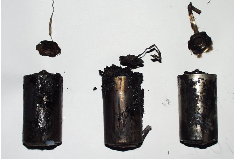
Figur 3.10. Cellene etter testing, LS 33600.
