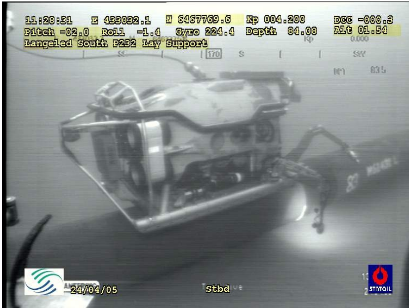
Figure 12.24 HiROV 3000 from Deep Ocean inspecting a pipeline. The DVL can be seen on the aft of the ROV.
