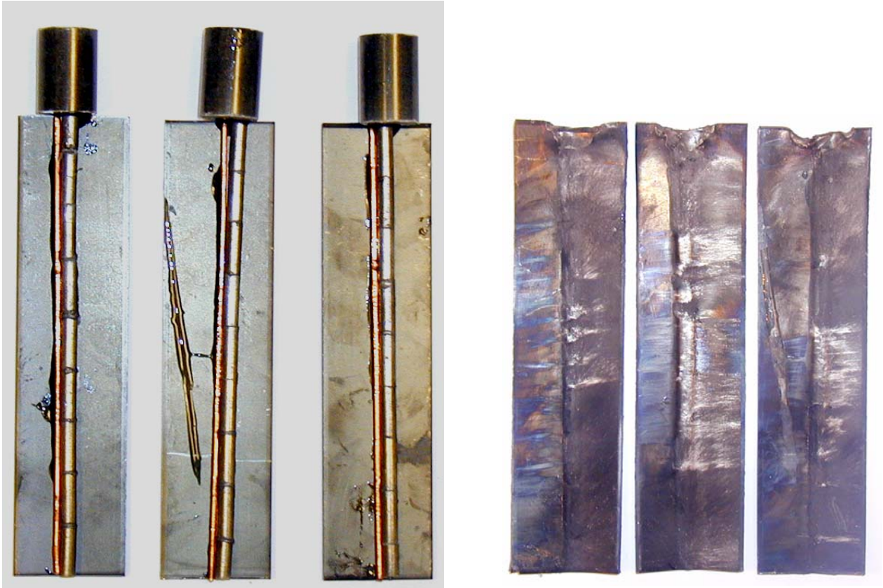
Figure 3.4 Pictures of charges used for testing of critical diameter, charge diameter 5.03 mm. The left picture shows the charges before testing and the right picture shows the witness plates after the charges were initiated.
