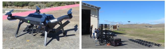
Fig. 16. Individual network-capable 3DR Solo drone (a); and a fleet of 20 networking UAS (b)
