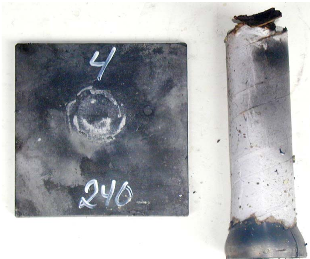
Figure 3.5 Shot No 4, tube No 4, barrier 240 cards, no reaction.
