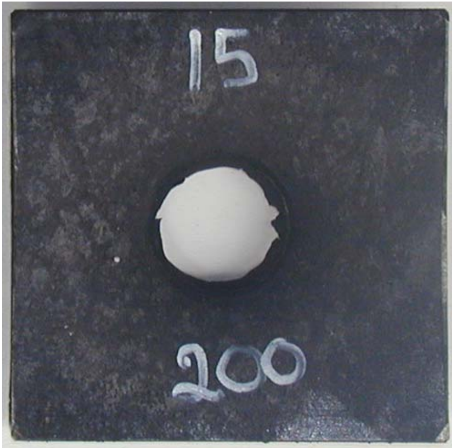
Figure 3.17 Shot No 15, tube No 15, barrier 200 cards, detonation.
