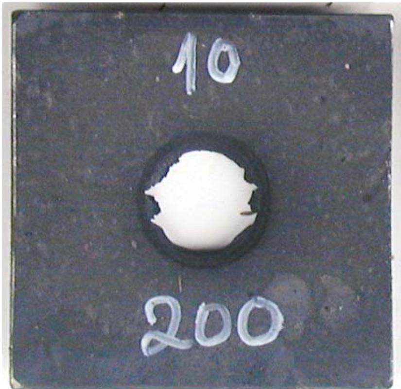
Figure 3.10 Shot No 9, tube No 10, barrier 200 cards, detonation.
