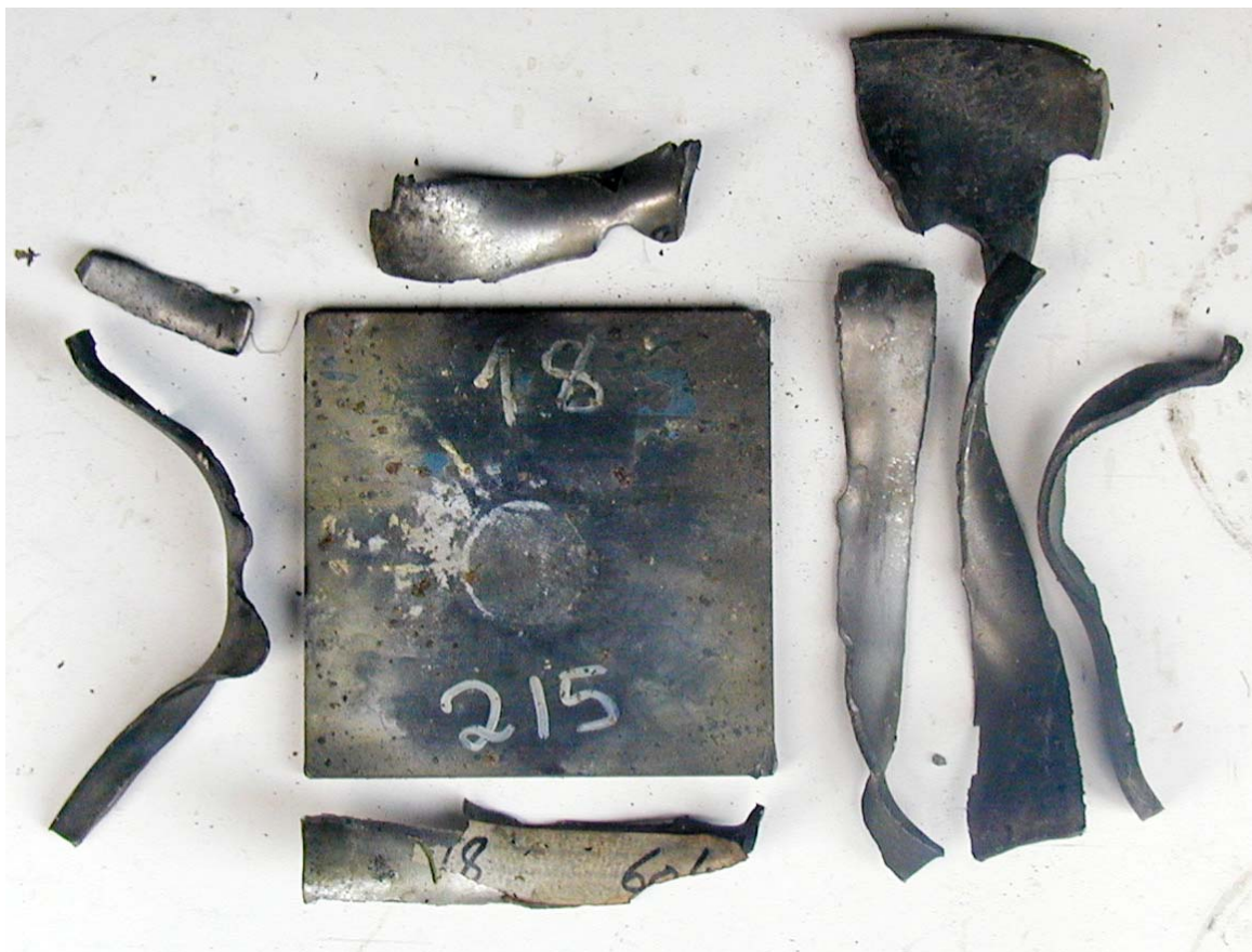
Figure 3.20 Shot No 18, tube No 18, barrier 215 cards, no reaction.
