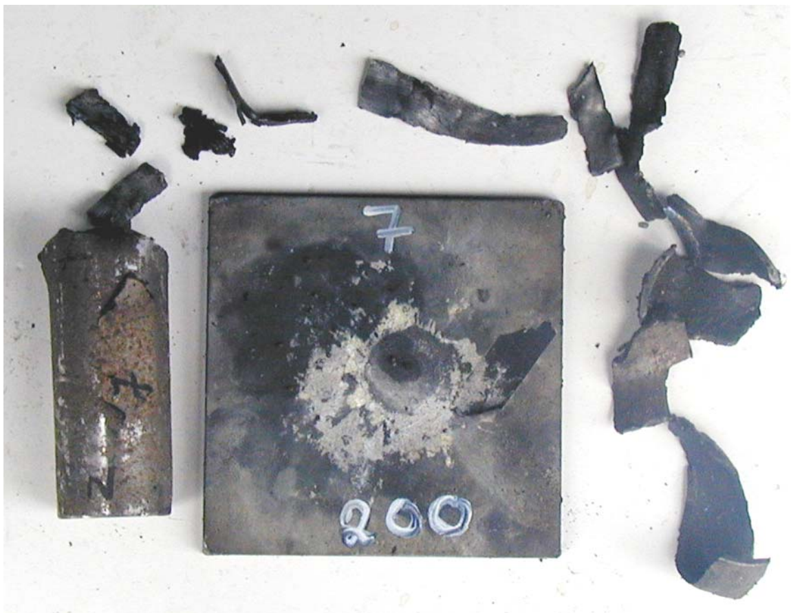
Figure 3.11 Shot No 10, tube No 7, barrier 200 cards, no reaction.
