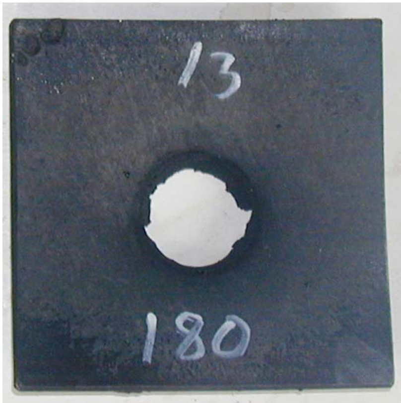
Figure 3.15 Shot No 13, tube No 13, barrier 180 cards, detonation.
