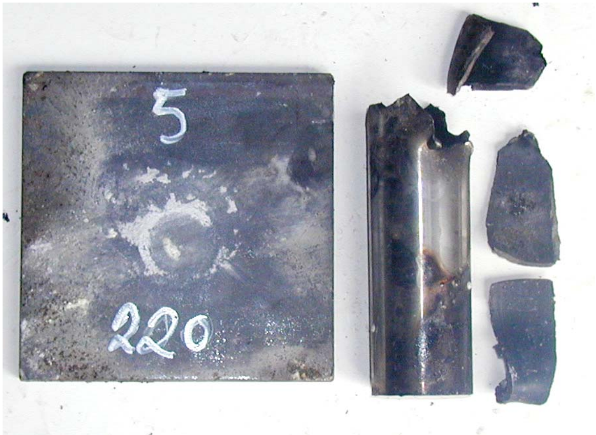
Figure 3.6 Shot No 5, tube No 5, barrier 220 cards, no reaction.
