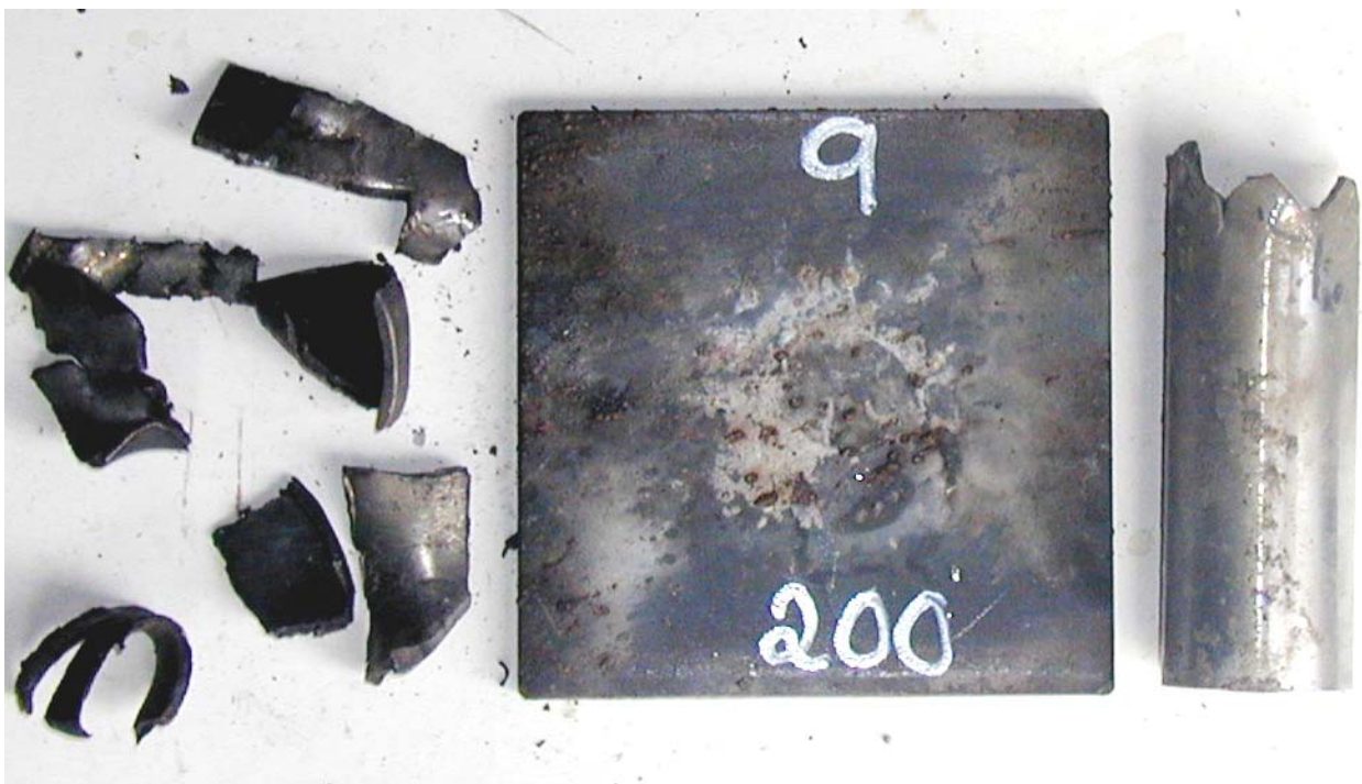
Figure 3.9 Shot No 8, tube No 9, barrier 200 cards, no reaction.
