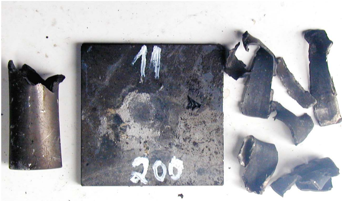
Figure 3.13 Shot No 11, tube No 11, barrier 200 cards, no reaction.
