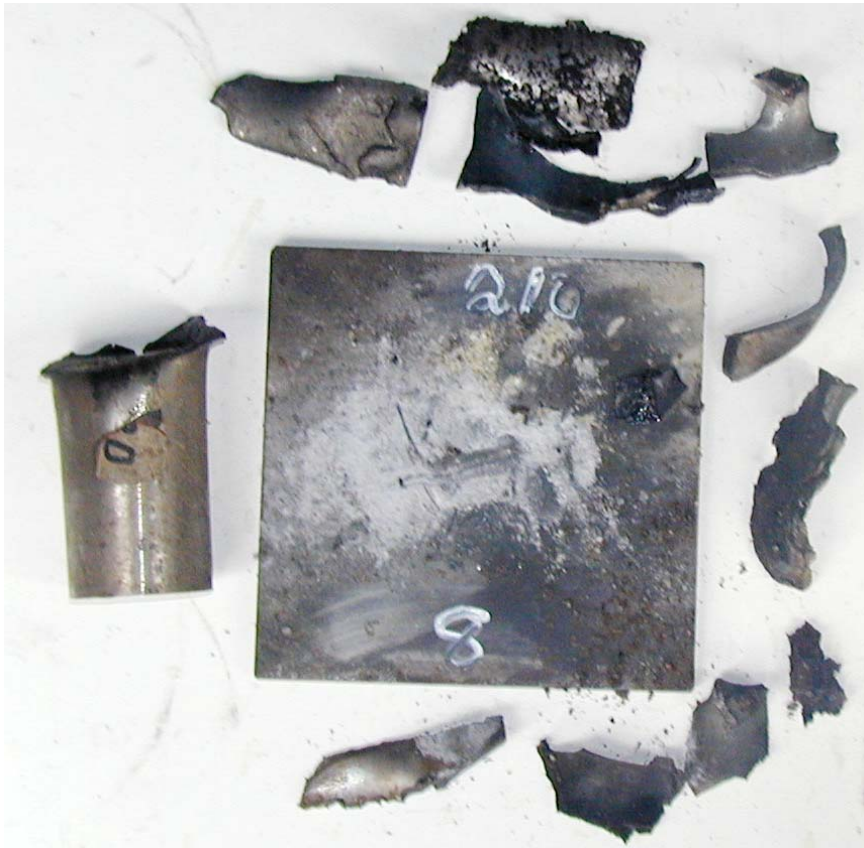
Figure 3.8 Shot No 7, tube No 8, barrier 210 cards, no reaction.
