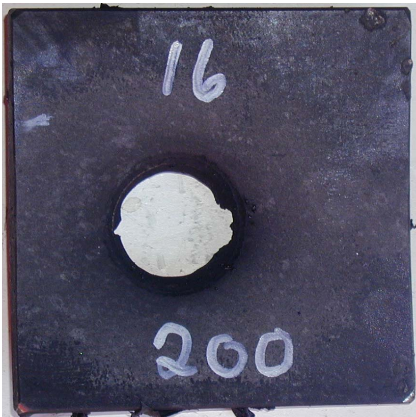
Figure 3.18 Shot No 16, tube No 16, barrier 200 cards, detonation.
