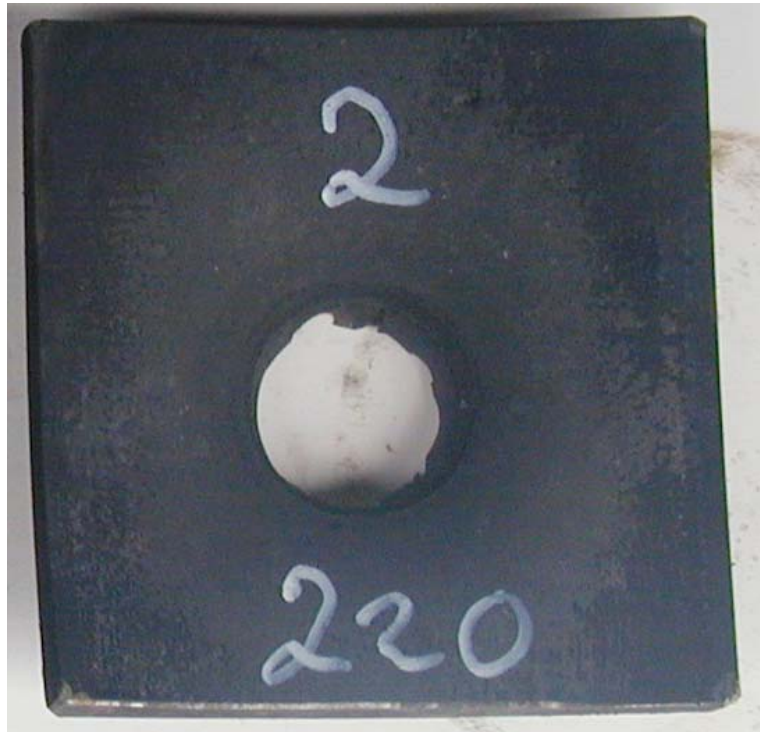
Figure 3.3 Shot No 2, tube No 2, barrier thickness 220 cards, detonation.
