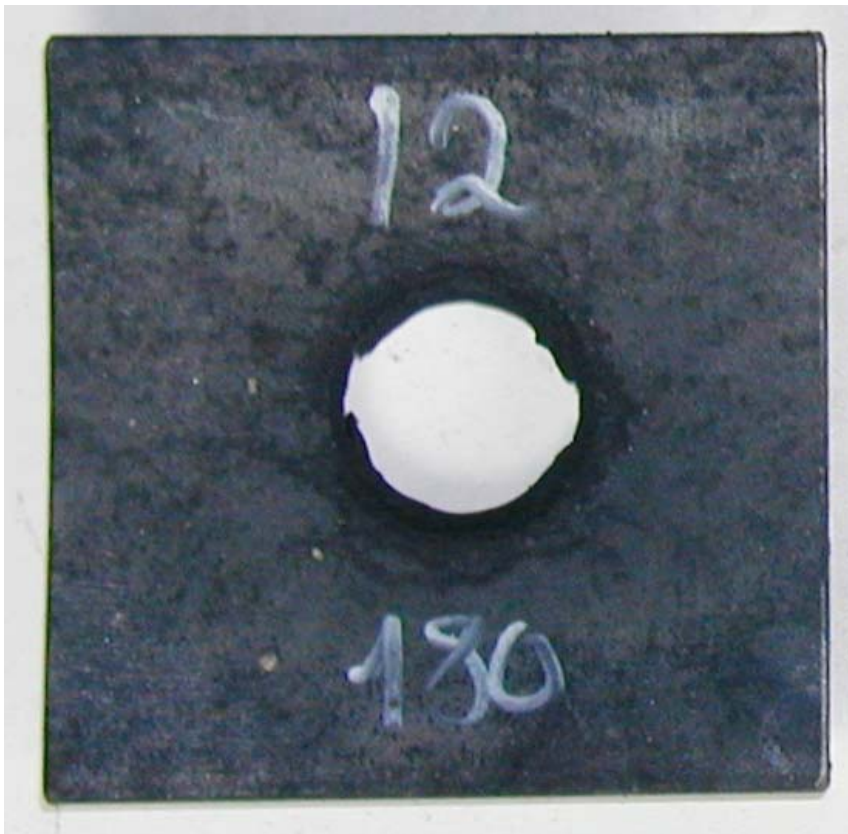
Figure 3.14 Shot No 12, tube No 12, barrier 180 cards, detonation.
