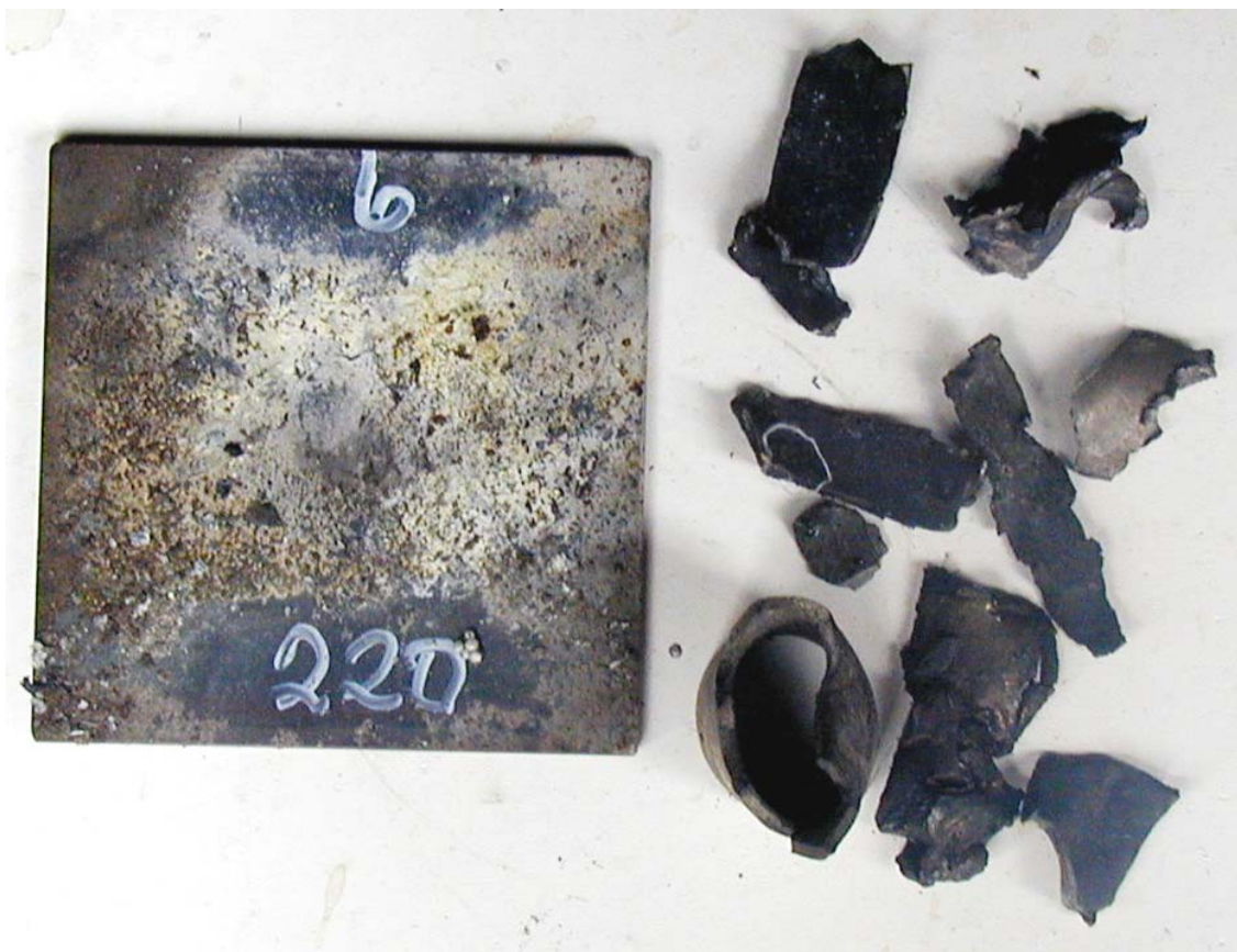
Figure 3.7 Shot No 6, tube No 6, barrier 220 cards, no reaction
