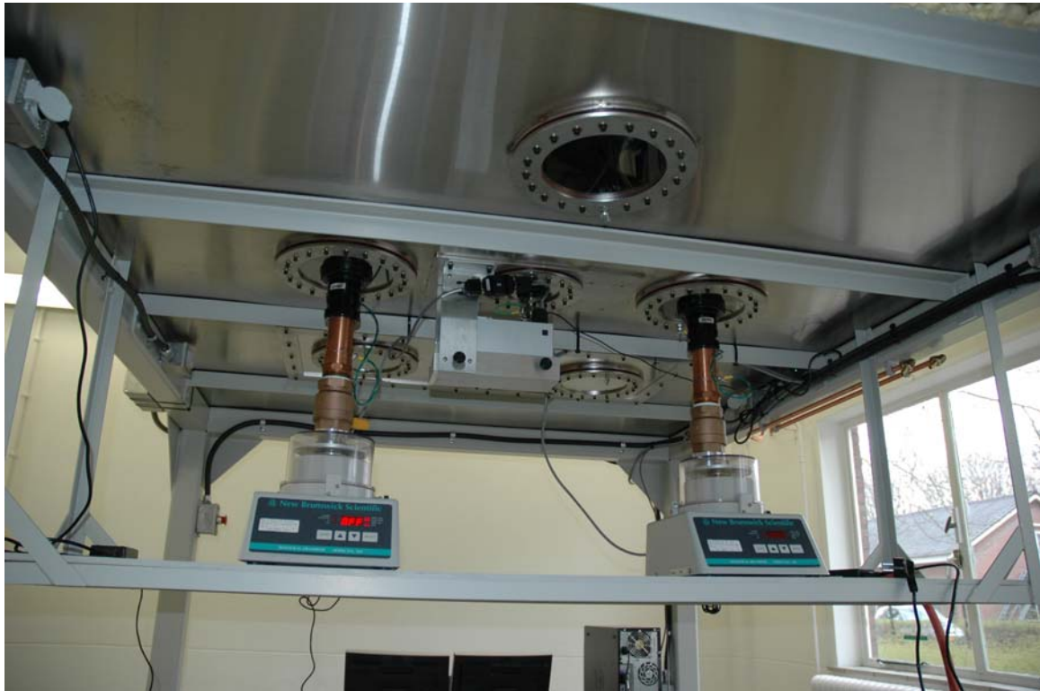
Figure 2.1 Connection of the slit-to-agar STA-samplers to the BAT chamber.
