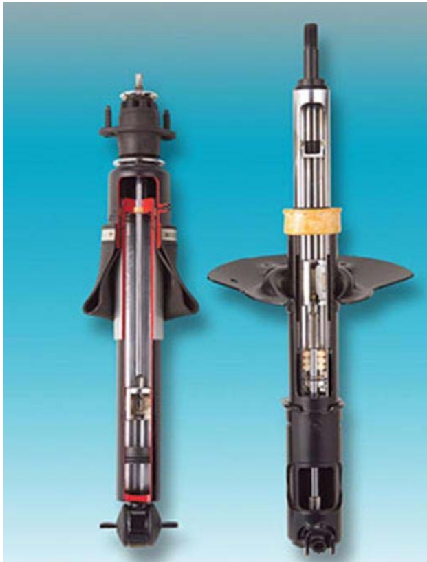
Figure 5.7 – Cutaway of rear shock absorber and suspension strut [11]
