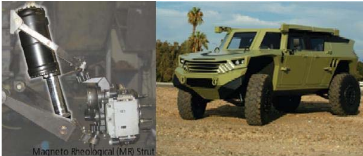
Figure 5.9 – Light utility vehicle with semi-active suspension [13]
