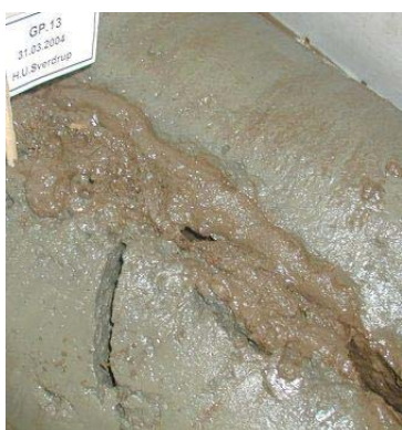
Figur A.7 Grab 13/04, 01.04.2004, 59°32,7450' N, 004°22,8352' E Clay and silt with sand and some gravel ( \leq 1 cm). Dark grayish brown color (2.5Y 4\2). Classification: Clayey silt with minor sand.
