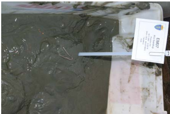
Figur D.5 Grab 05/07, "EM07", 14/11-07 12:09, 59°41.178' N, 3°07.840' E, 135 m Fine, silty sand. One small chunk of silty clay. Some biological material.
