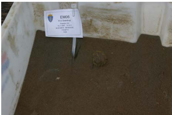
Figur D.6 Grab 06/07, "EM06", 14/11-07 13:13, 59°43.228' N, 3°00.413' E, 110 m Medium-fine sand. No silt or clay. Brownish-yellowish tint. A few shells and a nice sea porcupine.
