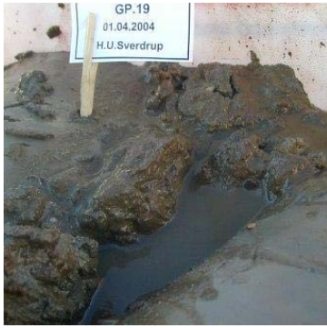
Figur A.11 Grab 19/04, 01.04.2004, 60°00,0570' N, 004°30,0154' E A mix of mud and coarser material. Lots of shell fragments. Dark grayish brown color (2.5Y 4\2). Classification: Sandy-clayey sand.
