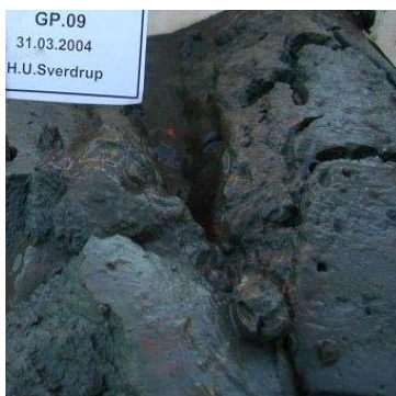
Figur A.4 Grab 09/04, 31.03.2004, 60°08.7702' N, 004°16.6771' E Sticky clay with silt and sand. Low water content. Some fine shell fragments. Dark gray color (5Y 4/1). Classification: Silty clay with minor sand.
