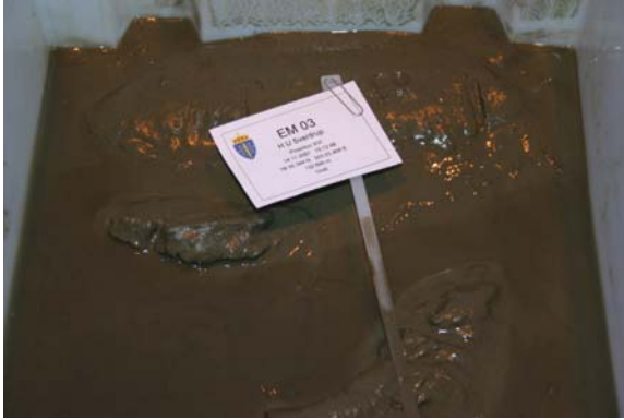
Figur D.7 Grab 07/07, "EM03", 14/11-07 15:12, 59°56.344' N, 3°05.468' E, 133 m Fine, silty sand. Olive greenish tint.
