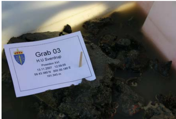
Figur D.1 Grab 01/07, "Grab 03", 13/11-07 12:59, 59°43.380' N, 5°00.180' E, 101 m, Silty sand and gravel with many pebbles and boulders (size 1-8 cm.). A few small shells. Very heterogeneous sample of glacial material (moraine).
