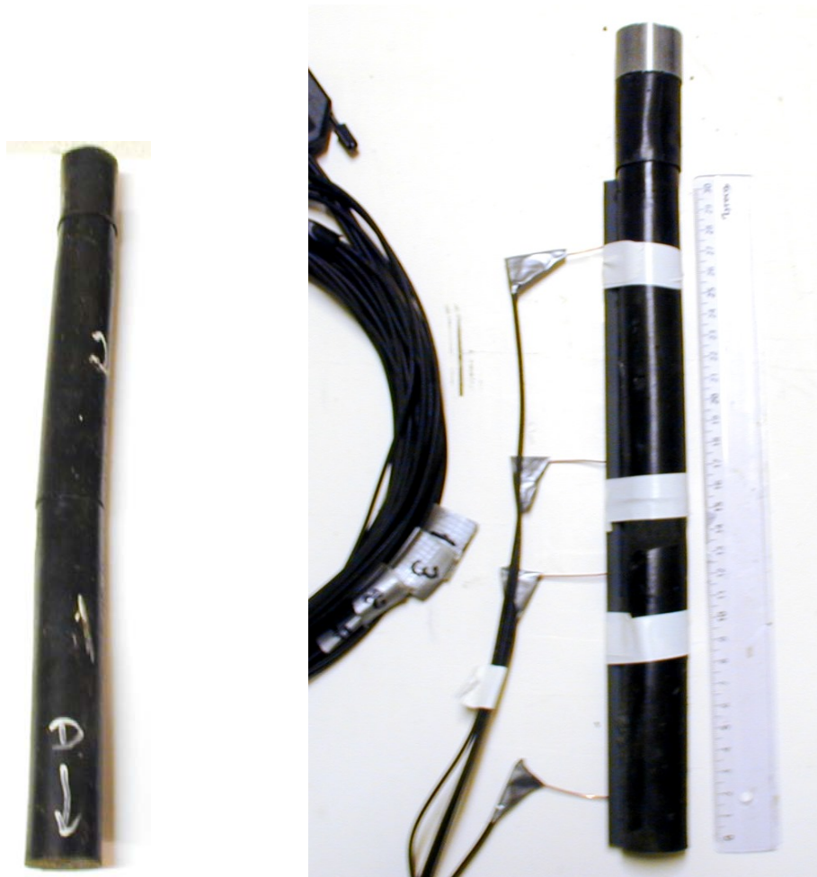
Figure 2.2 To the left the conglutinated test item, to the right the test item with ionization pins and booster added.
