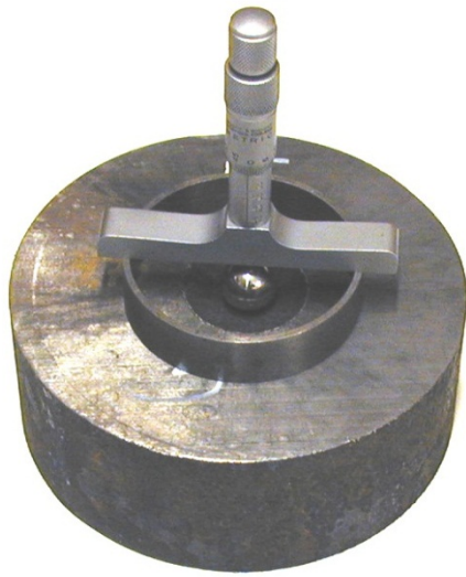
Figure 2.5 Picture of the tool used to measure the Dent depth.
