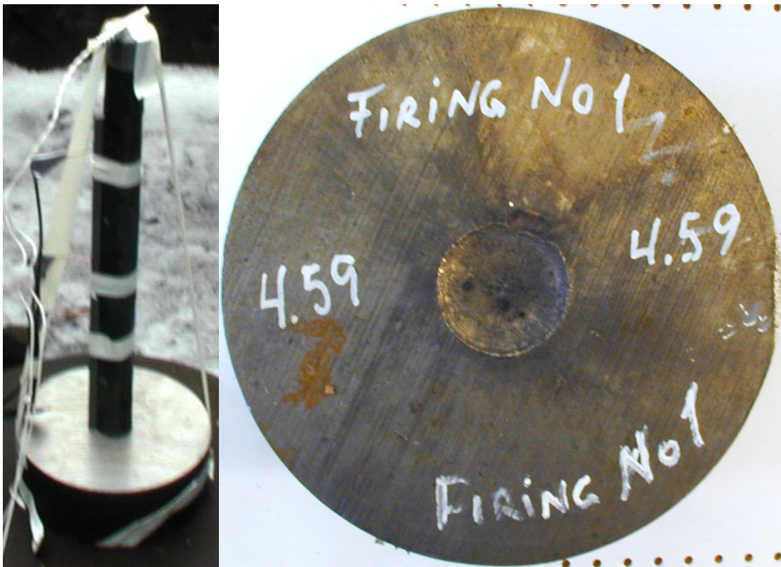
Figure 3.8 Test setup and the Dent plate for firing No 1 with cast No 1 (2).
