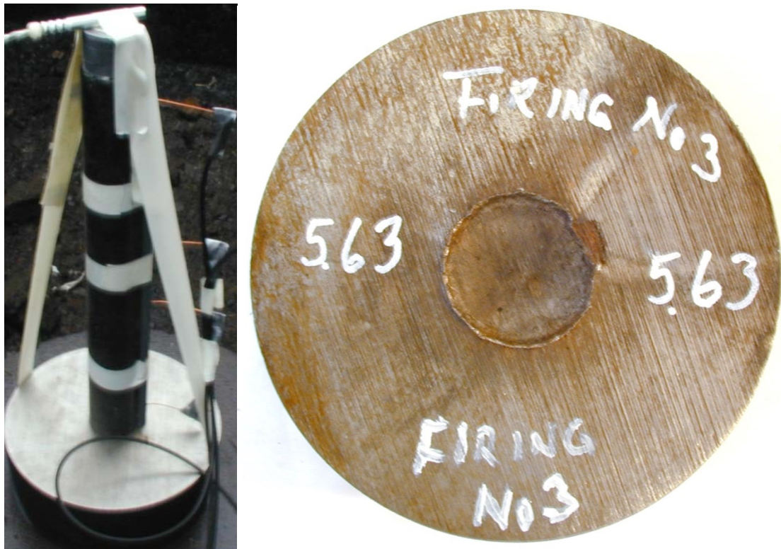
Figure 3.10 Test setup and Dent plate for firing No 3 with cast No 12.
