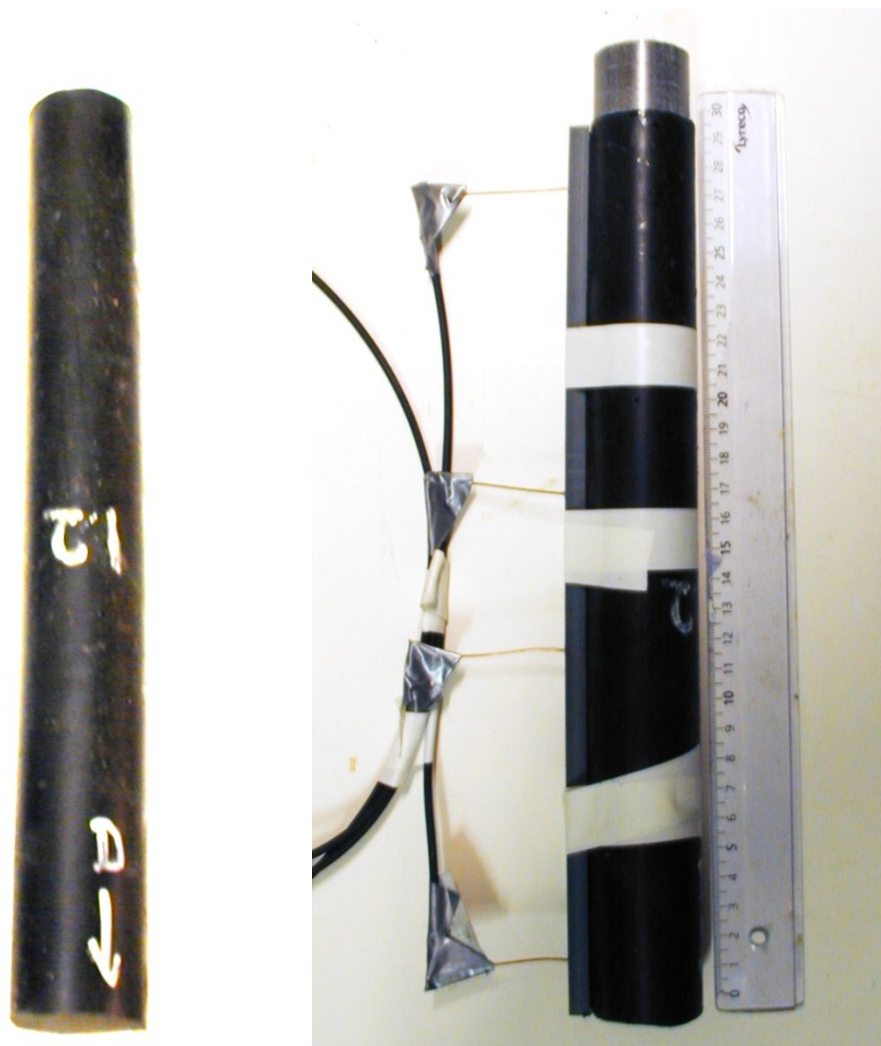
Figure 2.4 Pictures of test item 3 before and after addition of the booster and the ionization pins.
