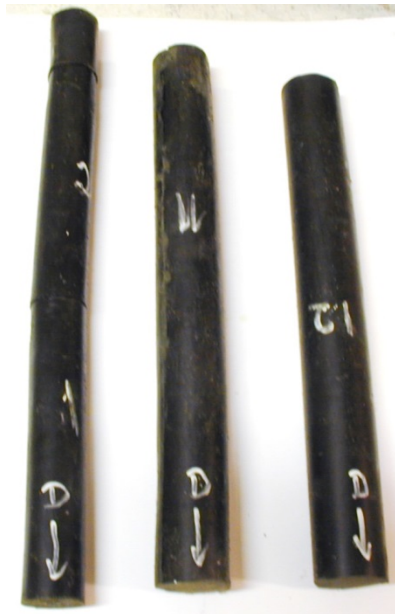
Figure 2.1 The charges to be tested with regard to detonation velocity and pressure.
