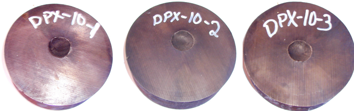
Figure 3.12 Picture of the Plate Dent witness plates for the DPX-10 shots.
