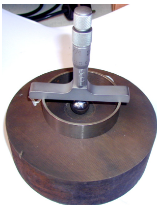
Figure 2.2 Picture of the equipment used to measure the Dent depth.
