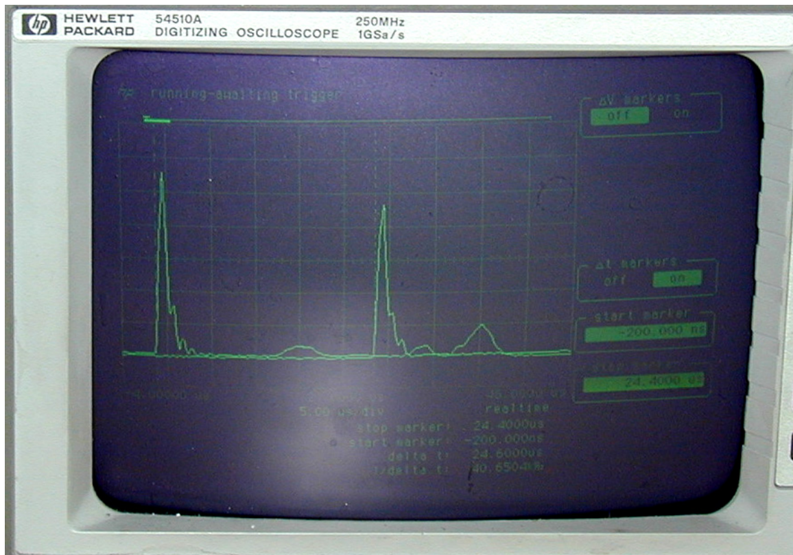
Figure 3.8 Picture of the oscilloscope registration for the second shot with DPX-10 sats 540/09.
