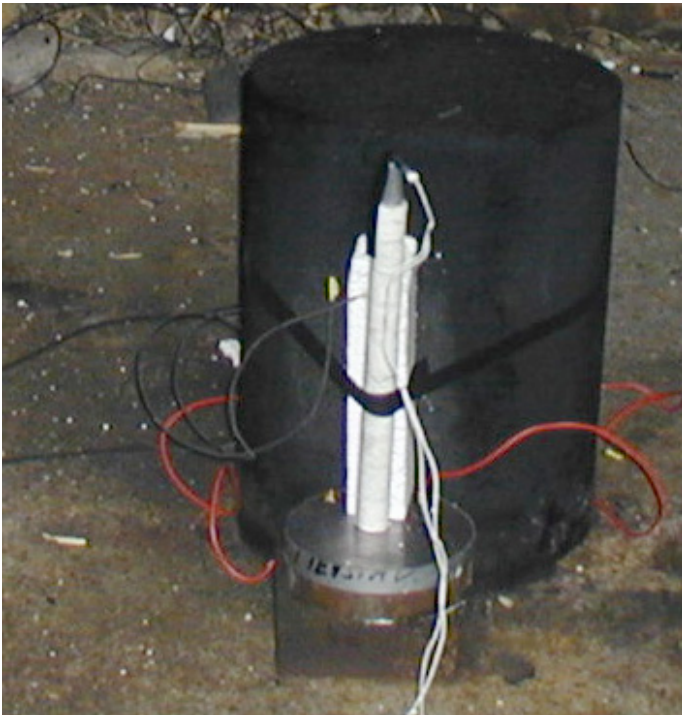
Figure 3.4 Picture of the test upset for shot 3 with DPX-9 sats 527/09 showing the Plate Dent witness plate at the bottom of the charge.
