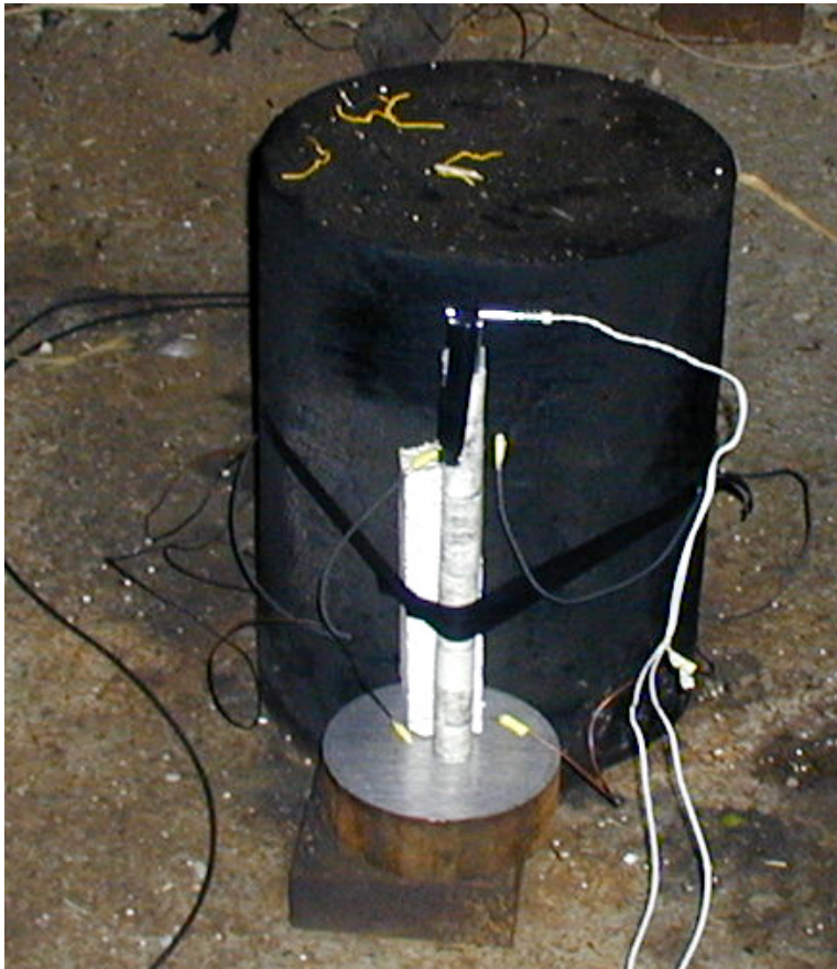
Figure 3.9 Picture of the test upset for shot 3 with DPX-10 sats 540/09 showing the Plate Dent witness plate at the bottom of the charge.
