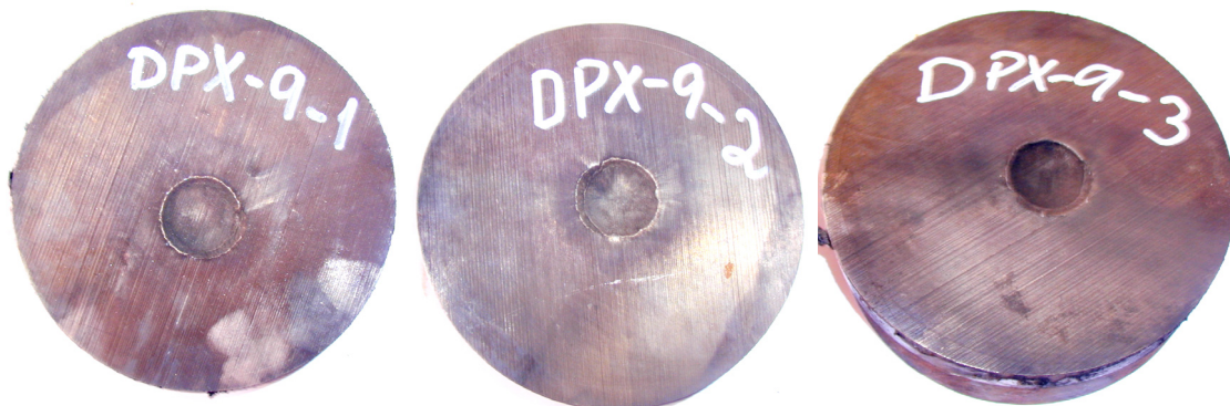
Figure 3.11 Picture of the Plate Dent witness plates for the DPX-9 shots.
