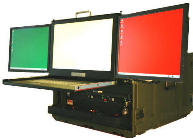
Figure 2.3 A DataVaultX4 tactical rugged mobile system [11].
