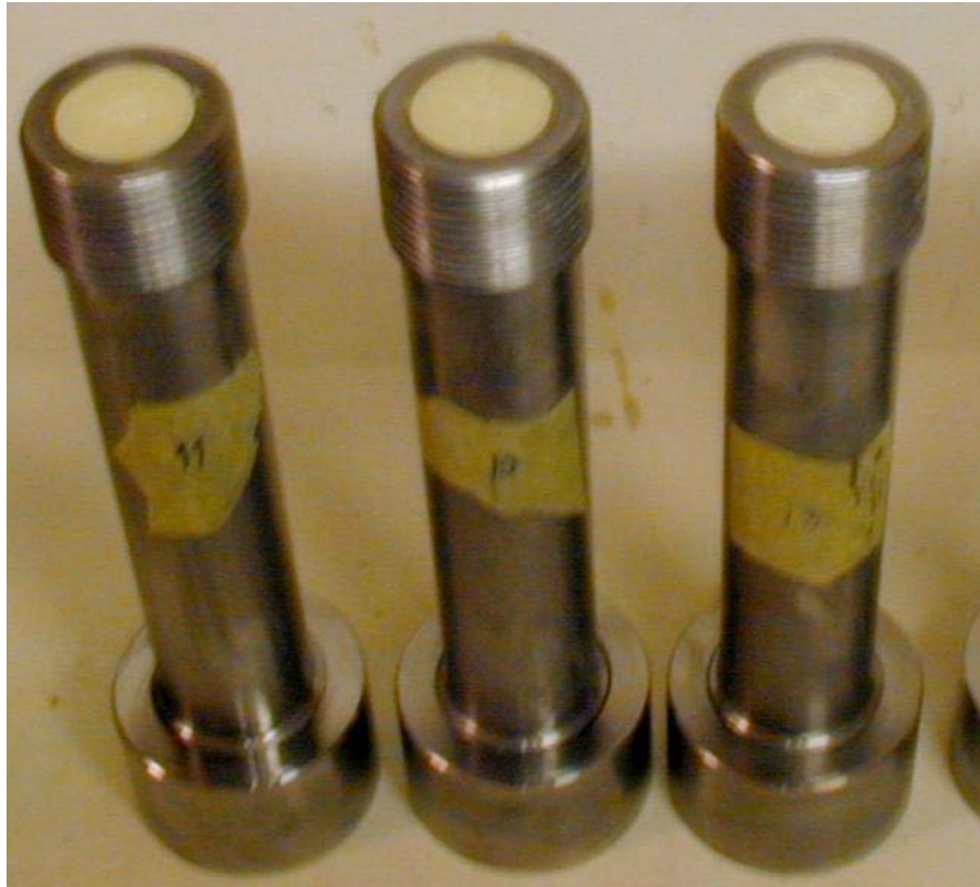
Figure 2.2 Tube No 11 to tube No 13 after cleaning and modification of the top surface.
