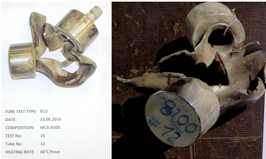
Figure 3.6 Recovered test vehicle No 12 after reaction in tube test No 18.
