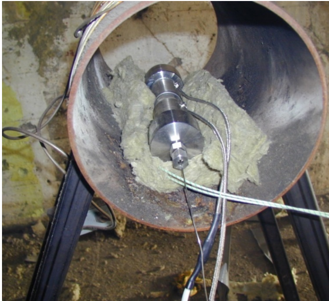
Figure 2.5 Picture of test item with the two heating elements and three thermocouples.
