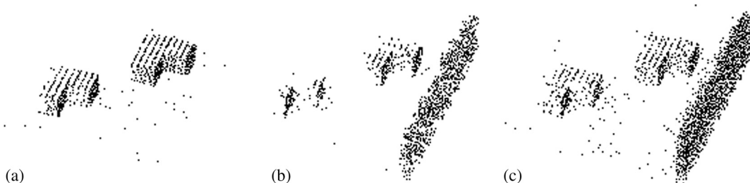
Fig 9 Point clouds of two buildings on a flat ground. To make the buildings clearly visible, only points above the ground level are shown. (a) Obscuring forest absent, detection threshold 1 and FOM threshold 11 (automatic). (b) Forest present, same parameters as in (a). (c) Forest present, FOM threshold 4 .
