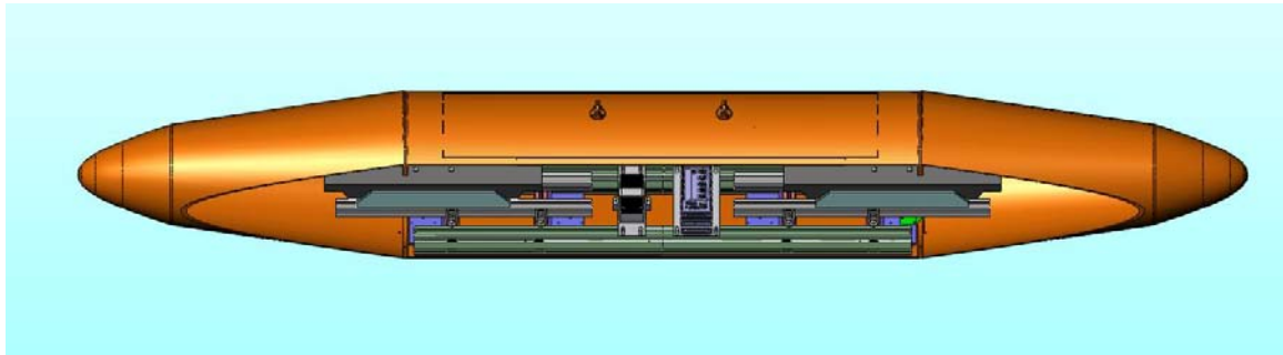
Figure 4.3 Cross section of the MXU-648A/A with the lead weights distributed. The distance between the weights can be adjusted incrementally from zero to the outer position as shown in the figure.
