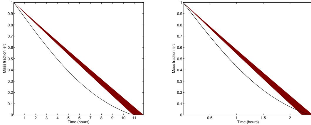
Figure 5.1 Mass fraction left as function of time. The FFI model results are shown as full line. The coloured area is the range given by the ADVEDS model with a slip velocity in the range explained in the text. The figure on the left is for a droplet with volume  $V = 1 \mu\text{l}$ , temperature  $T = 15^\circ\text{C}$  and bulk air velocity of  $U = 1.77 \text{ m/s}$ , while the figure on the right is for  $V = 1 \mu\text{l}$ ,  $T = 35^\circ\text{C}$  and  $U = 1.77 \text{ m/s}$ .
