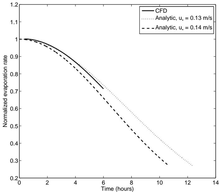
Figure 4.1 Normalised evaporation rate calculated with the UDF for RANS simulations and analytically as function of time.
