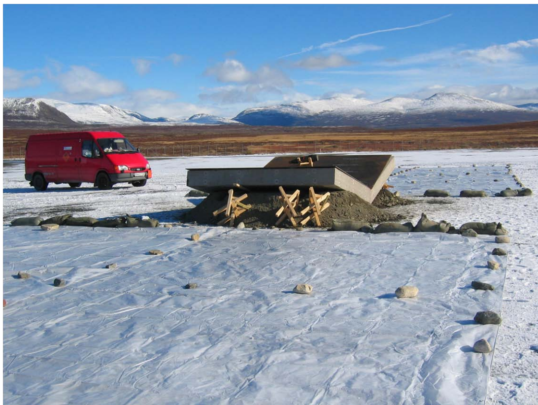
Figure 1 Sampling of explosive particles from a low order detonation of a 155 mm grenade at Hjerkin, Norway.
