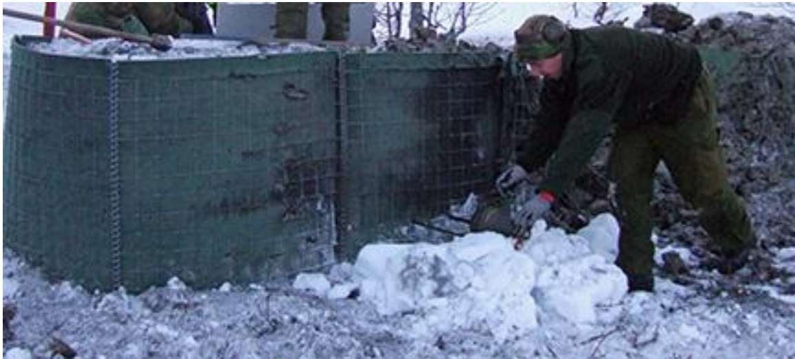
Figure 2.6 Position of 3.5 kg shaped charge in test 1.5
