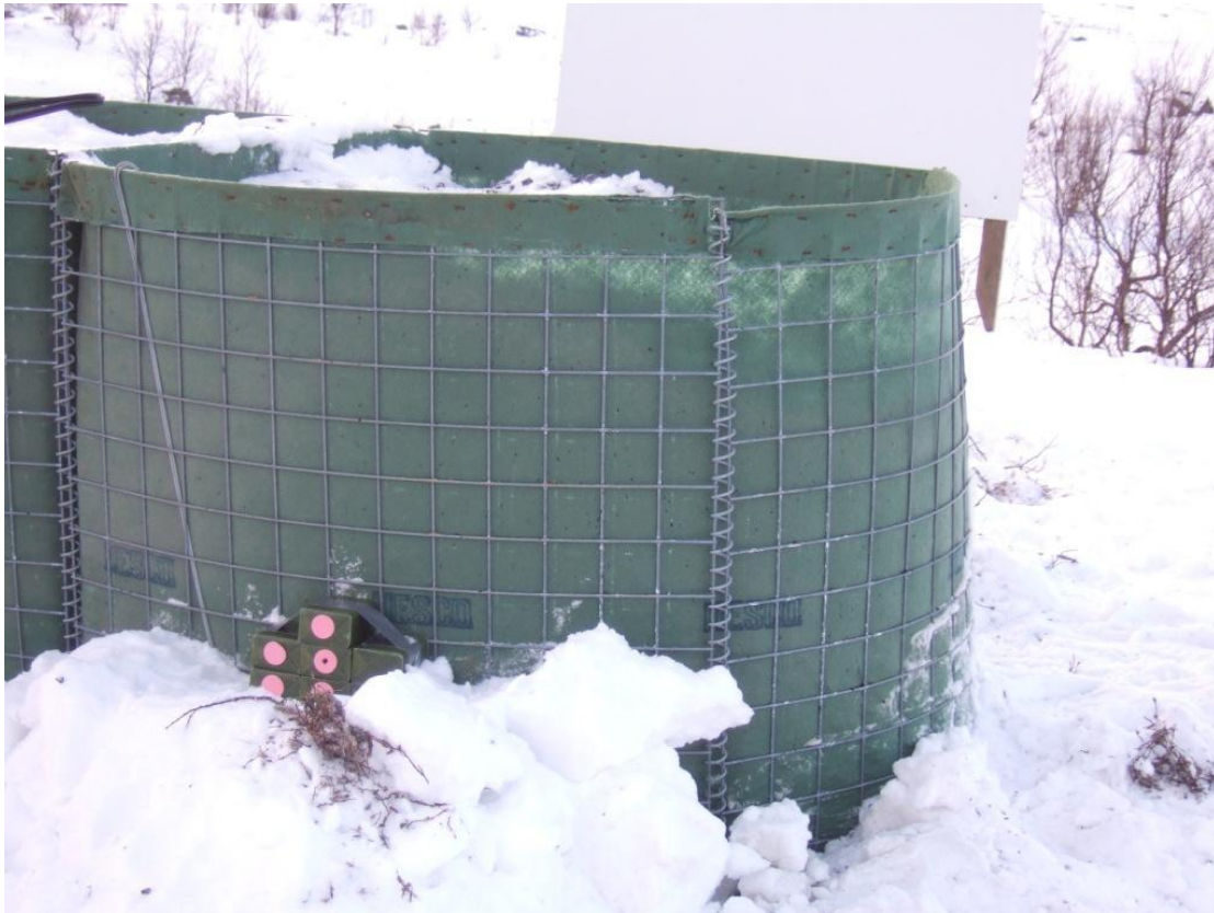
Figure 2.2 Setup of test 1.1 with 3.5 kg TNT
