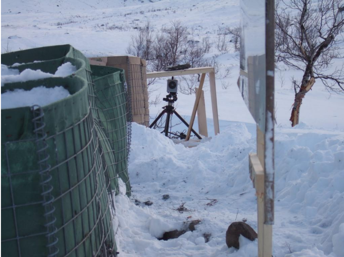
Figure 2.1 High-speed video camera used in test 1
