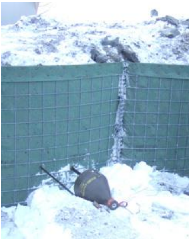
Figure 2.5 3.5 kg shaped charge in test 1.4
