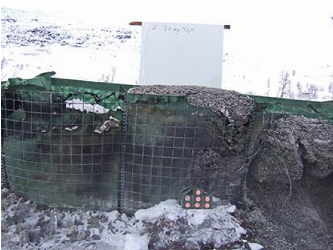
Figure 2.3 Setup of test 1.2 with 7.0 kg TNT
