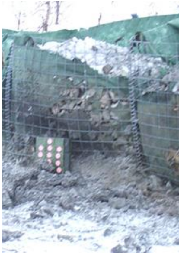
Figure 2.4 Setup of test 1.3 with 7.5 kg TNT
