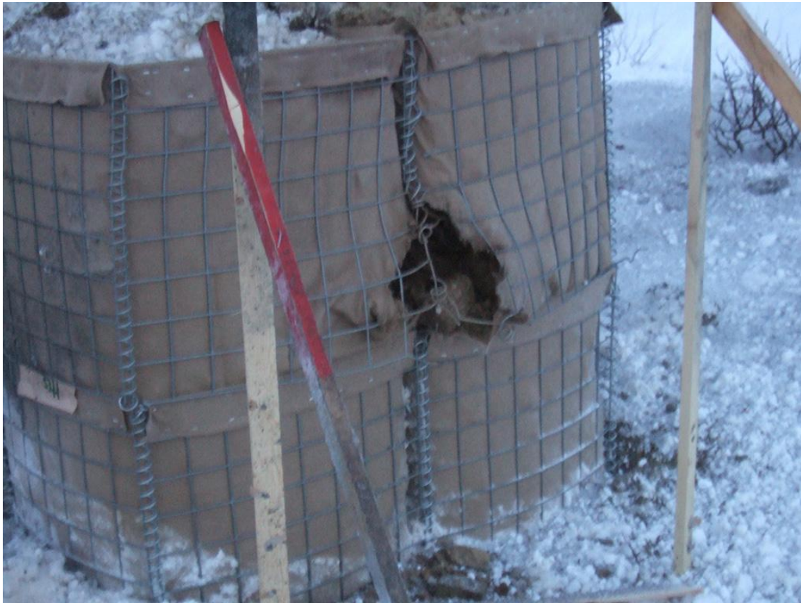
Figure 2.17 Back side of wall after test 1.6
