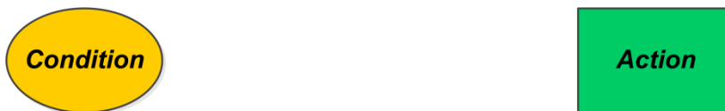
Figure 4.6 Graphical representation of the condition node (to the left) and the action node (to the right). The “ Condition ” and “ Action ” text labels will typically be descriptions of the condition and the action respectively.
