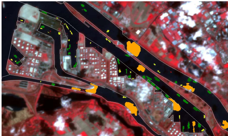
Figure 16. Filtering of clouds (orange) and noise (red) from large ships (dark green) and small ships (light green)
