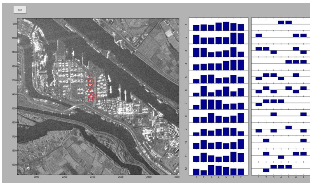
Figure 115 Interface of the multi-temporal change detection tool showing temporal behaviour of oil terminal content.
