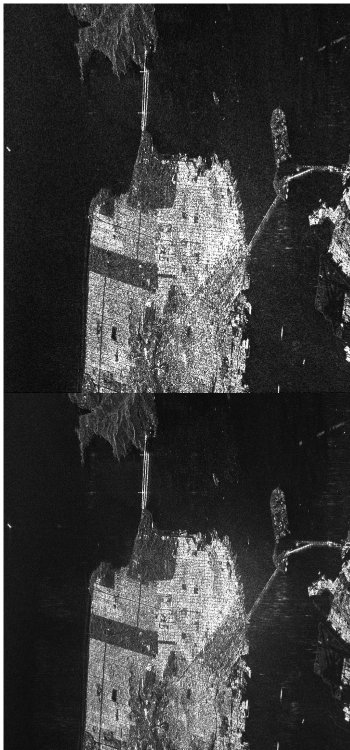
Figure 49. Top: DCP double bounce simulation (HH-VV). Bottom: Quad-polarisation double bounce (HH-VV).
