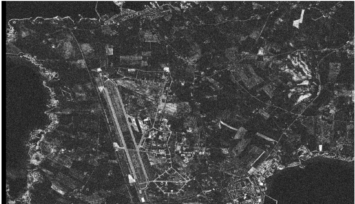
Figure 28 Coherence image from TerraSAR-X image pair for Ørland airbase.
