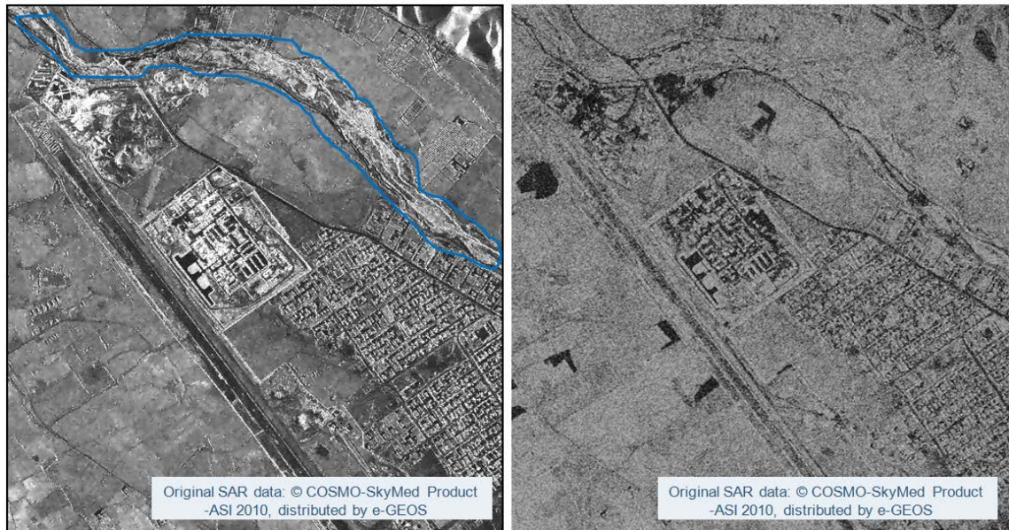
Figure 24 Amplitude and coherence image from COSMO-SkyMed image pair for Meymaneh city in Afghanistan.
