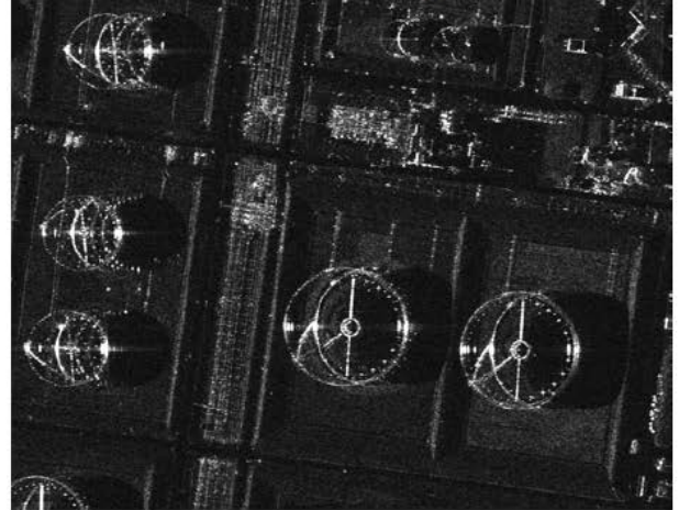
Figure A.44 TerraSAR-X images of Rotterdam harbour showing oil drums. A comparison between HS and ST modes is shown.
