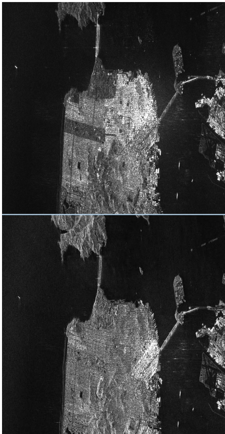
Figure 51. Top: DCP volume simulation (HV). Bottom: Quad-polarisation volume (HV).
