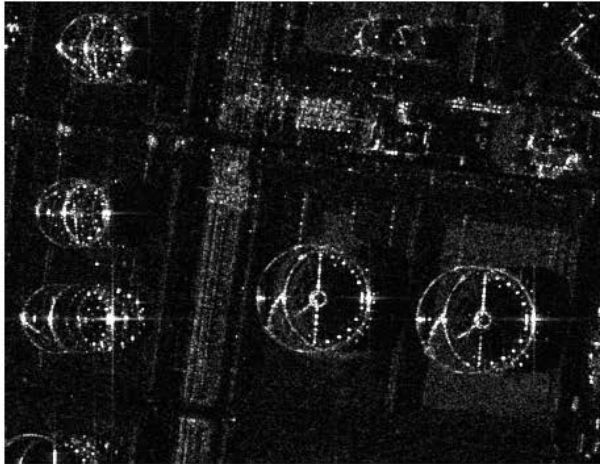
Figure A.44 TerraSAR-X images of Rotterdam harbour showing oil drums. A comparison between HS and ST modes is shown.
