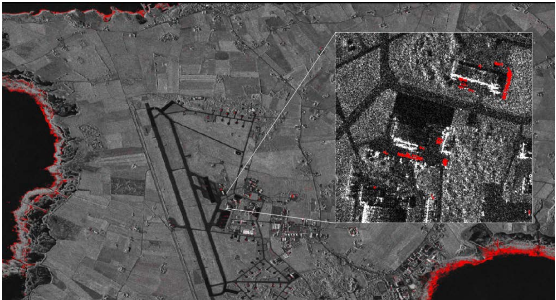
Figure 23 TerraSAR-X images (15 and 26 June 2013) for the Ørland area (courtesy Fraunhofer IOSB) with changes due to tide and relocatable vehicles (red overlay).
