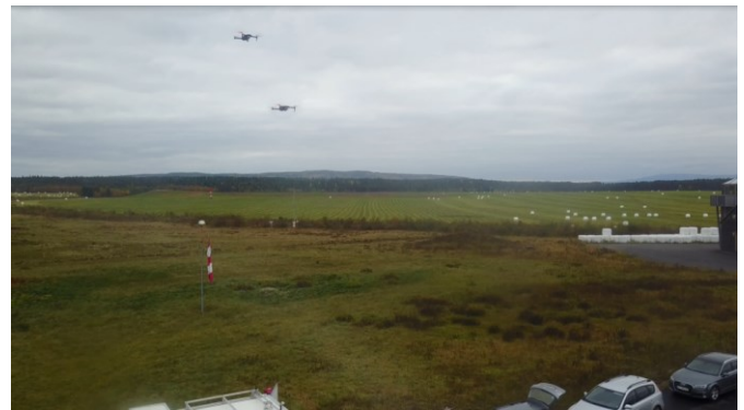
Fig. 3 Two DJI Mavic Pro drones meeting at the rendezvous point before the spent drone returns to base and the fresh drone continues the ISR operation.
