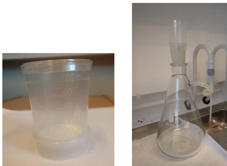
Figure 2.2 Filtration of water using the membrane filter method and vacuum support. (Photo: FFI)
