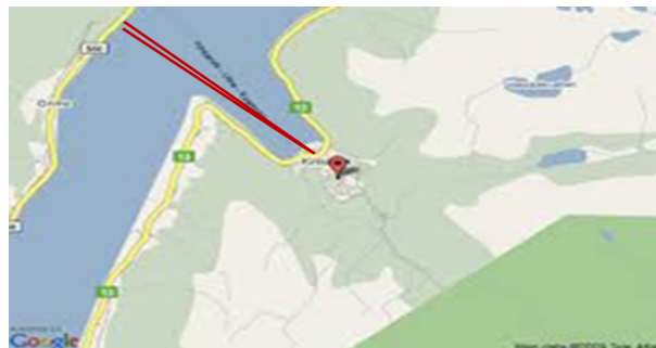
Figure 5.3 Since the distance between the ends of the curve after a back-and-forth crossing is very small, a ro-ro ferry has a high arch-curve ratio.
