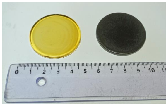
Figure 1. Examples of a neat epoxy sample (left) and a graphene/epoxy composite sample (right).
