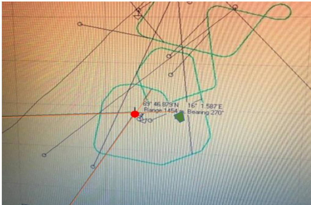
Figure 3.16 Example of target motion analysis on the logger display using the VHF signal from the tag and the DF-Horten directional receiver. A cross-bearing position (red dot) was made based on two bearings (orange lines) made before and after a turn of the ship (green line). This was considered to be a rough position of the focal whale, and based on this we could guide the acoustic tracking to choose the correct acoustic track of the focal whale, and set up the geometry of night time exposure experiments.
