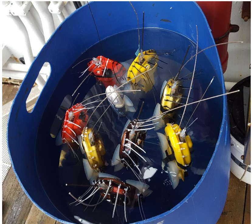
Figure 3.24 Testing the buoyancy of the 8 Mixed-DTAGs and 1 standard DTAGv3 that were available for the trial.
