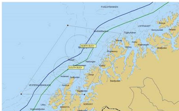
Figure 12. Intended mooring locations for acoustic recorders with 20nm range rings. Indicated is also the general operation area. The planned positions of the moored buoys are: 70°00.000N / 016°30.000E
