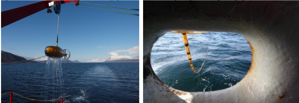
Figure 2. The sonar source SOCRATES (left) and acoustic array Delphinus (right) safely recovered on the
