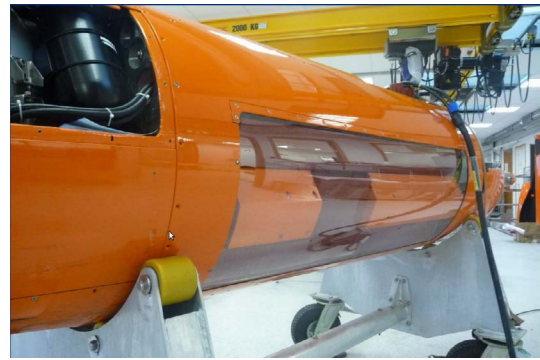
Fig. 2. The HISAS 1030 wideband interferometric SAS.
