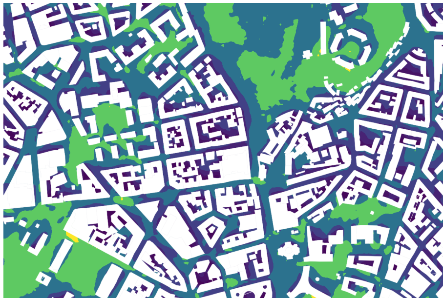
Figure 8.9 Turbulence kinetic energy in the same region as Figure 8.3 (also marked by red, dashed lines in Figure 8.2). Data taken from the 200° global-wind simulation. Contour levels range from \lesssim 0.03 (dark blue) to > 1 (yellow) \text{m}^2/\text{s}^2 and the energy doubles at every successive level.
