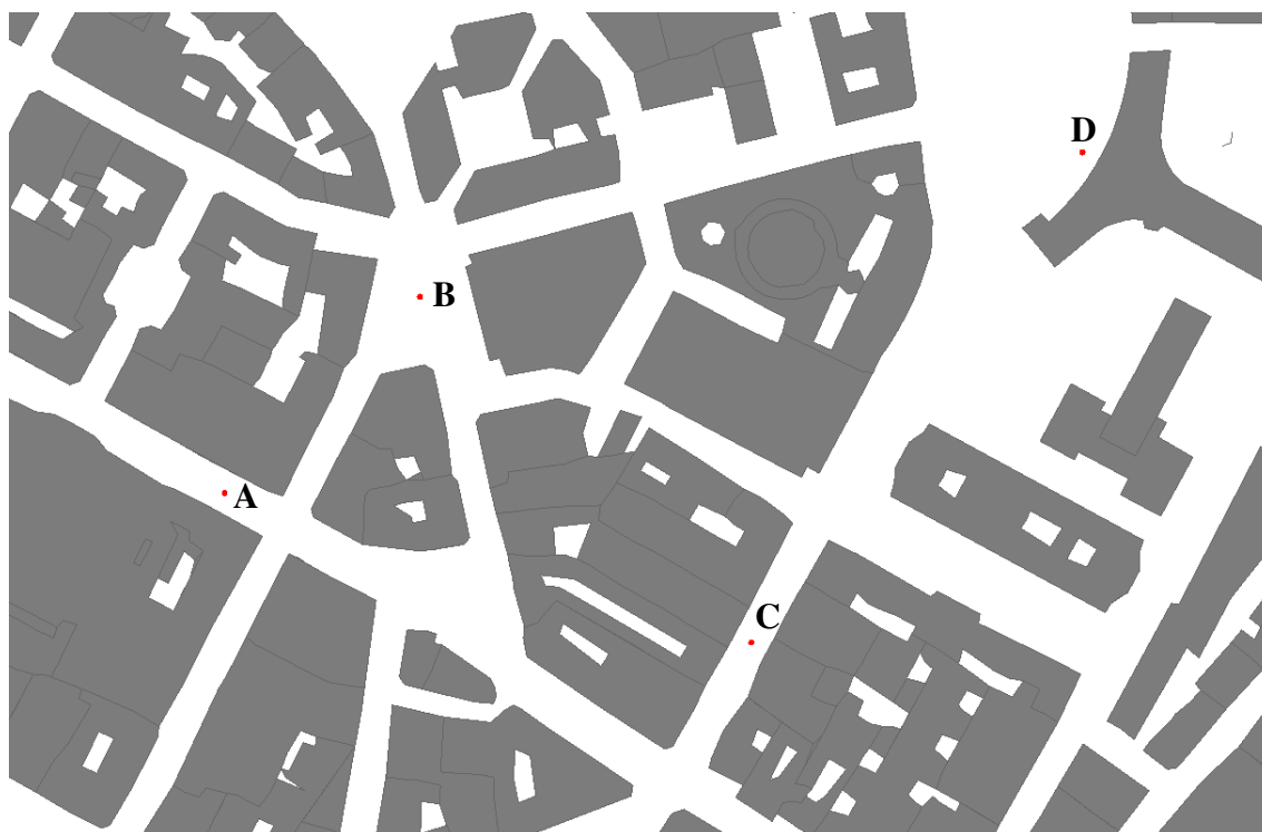
Figure 6.3 A portion of the mesh-study subdomain, along with the locations (shown as red dots) of the vertical profiles (A-D) shown in Figure 6.4 and Figure 6.5.
