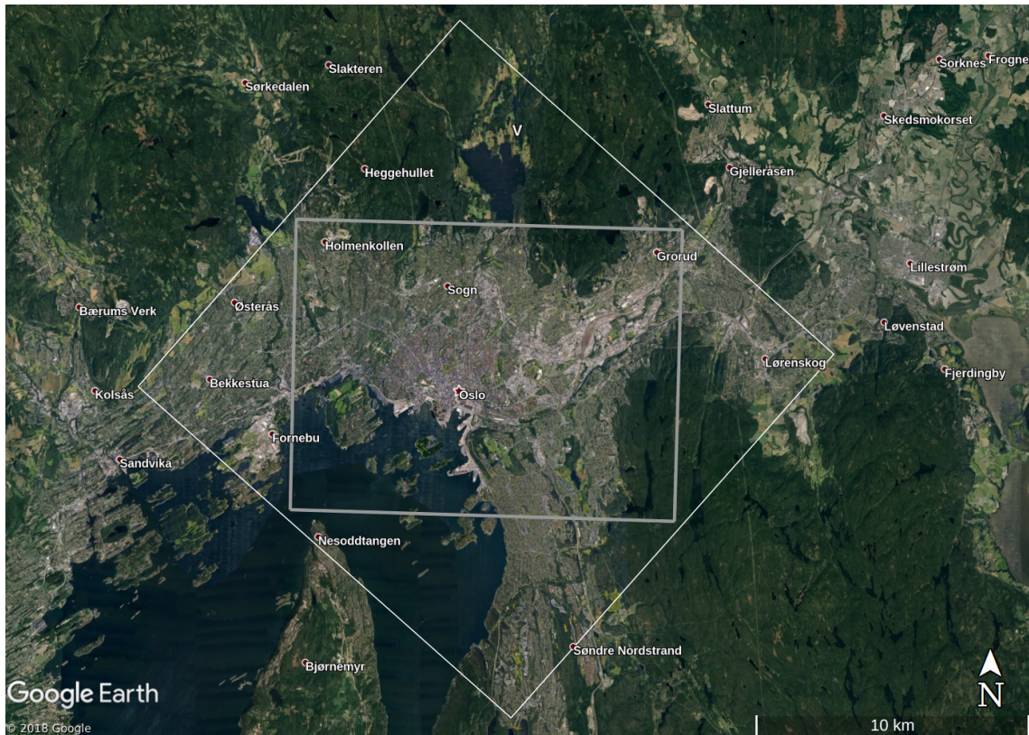
Figure 6.1 The geographical area of interest, shown as a grey rectangle in Google Earth. The dimensions of the area are 14.5 \times 11 \text{ km}^2 . The larger white rectangle shows the computational domain for the 40^\circ meteorological-wind simulation.
