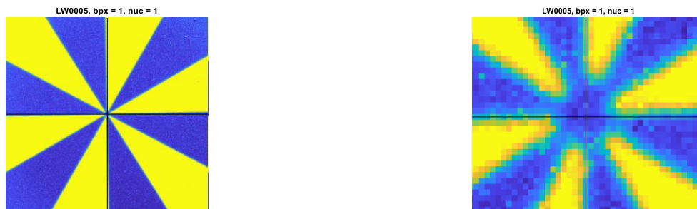
Figure 2. Example of a recording (here LW) of the Siemens star (left) and a zoomed-in version (right) to show details about the center of the recording. The cross hairs indicate where the center of the star is. In this case, the minimum circle radius is 6 pixels and this corresponds to the highest spatial frequency that can be considered in his recording.
