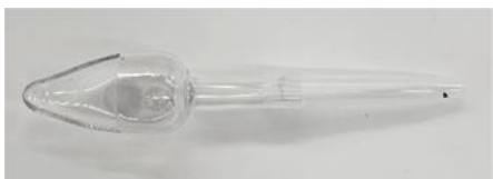
Figure 2.5 Weighing funnel used to transfer the NMC material to the tube.
