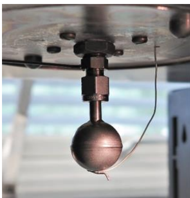
Figure 2.4 Setup for the electrolyte ARC test.
