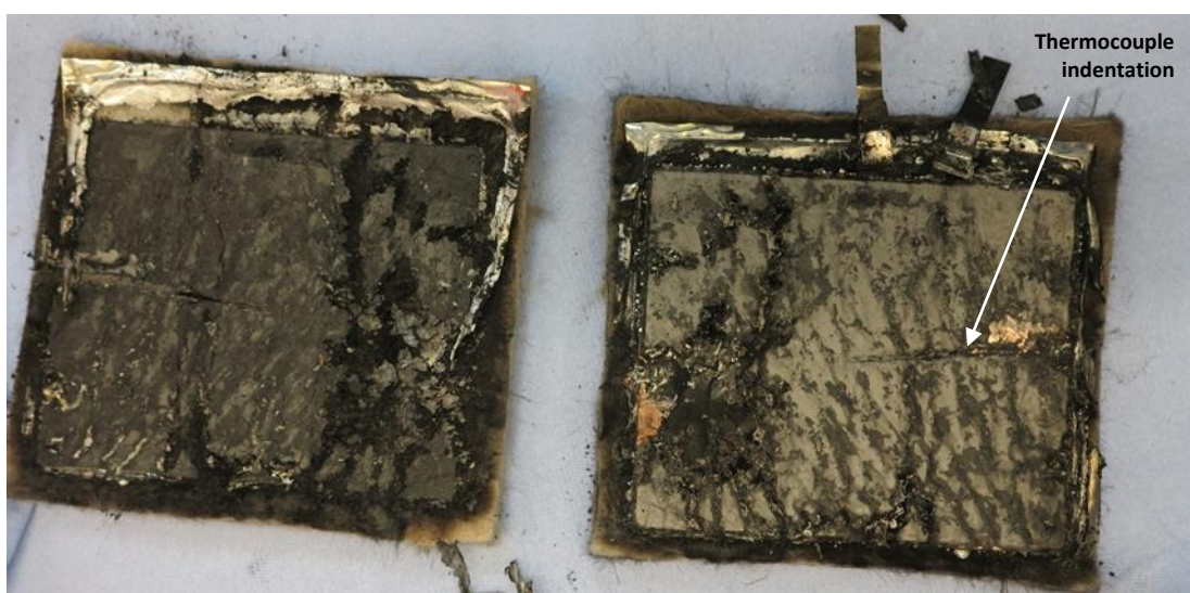
Figure 4.9 Photograph of the cell front post thermal runaway. The part on the left is the melted Al pouch stuck to the Pyrogel insulation material. The rest of the cell is on the right.
