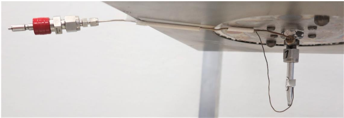
Figure 2.7 Side branch setup (2). The side branch was connected to the external gas fixture.
