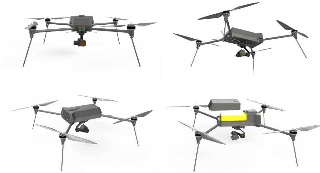
Figure 3.4 Flamingo viewed from different sides. Battery in yellow showed under cover.
