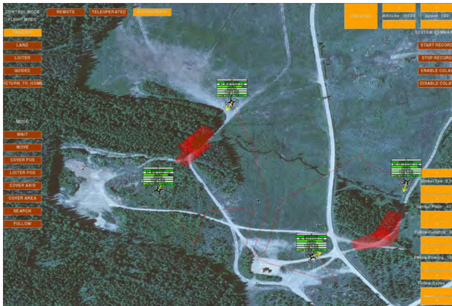
Figure 4.1 Snapshot of control station showing four drones covering two axes from different angles
