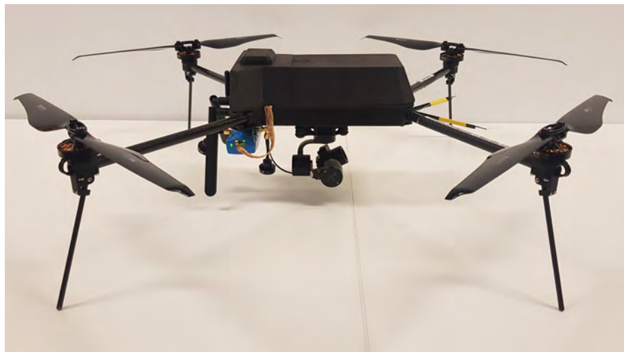
Figure 3.2 Flamingo with a mesh-radio and thermal camera.
