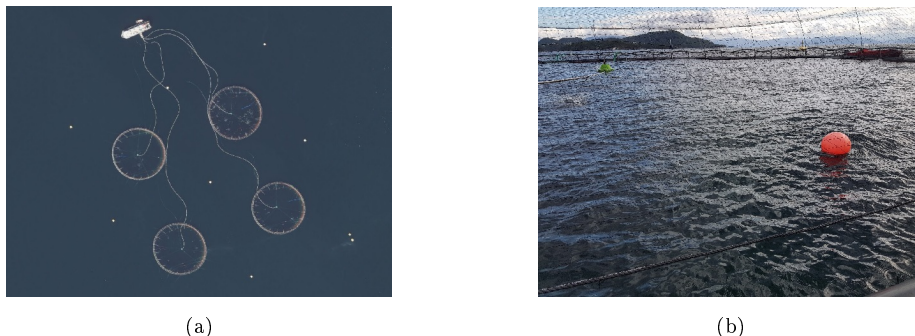
Figure 1: a) Aerial photo of the location, the pen in the upper right was used for the measurement. The pipes visible in and around the pens was used for pellet transportation. (Photo courtesy of Norge i bilder, Kartverket, Geovekst og kommunene.) b) Photo of the measurement site, the transmitter-receiver pair was suspended from the red buoy. A jumping salmon is noticed in the upper left of the photo.
