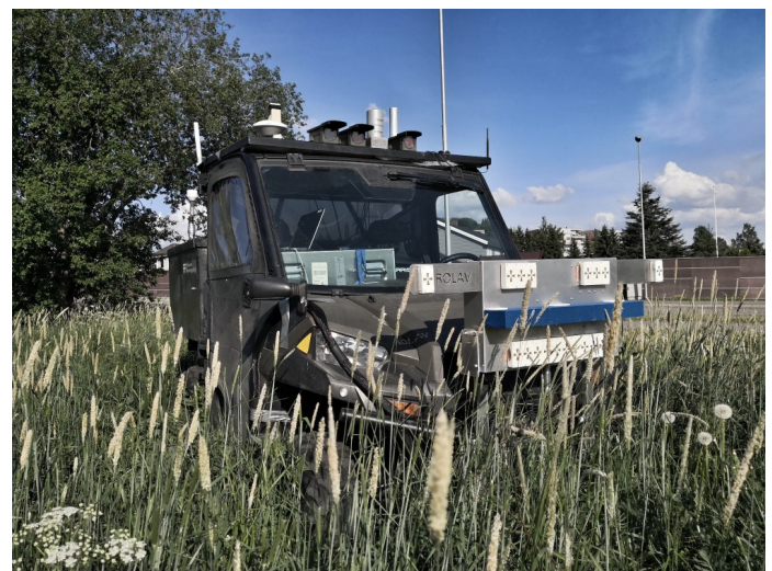
Fig. 12: OLAV platform in heavy vegetation with radar mounted in front.
