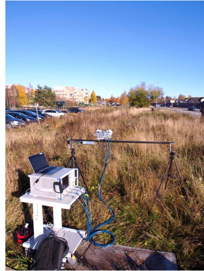
Fig. 3: Image of the measurement setup for target contrast measurements, the targets are hidden in vegetation.
